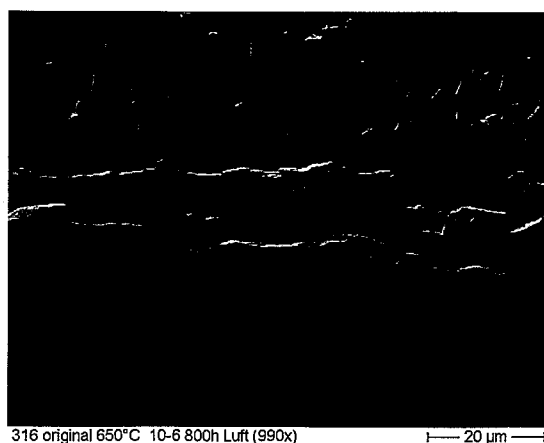
Fig. 54: 316 FR after 800 h oxidation in furnace atmosphere at 650 °C
