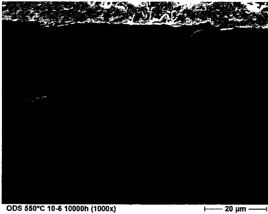
Oxide scale on ODS steel after 10000 h of exposure – near LBE surface – top of crucible
