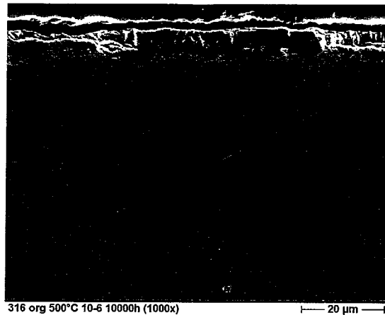
Fig. 3: Surface part of 316 FR steel without dissolution attack after 10000 h exposure at 500 °C. Note the oxide scale observed at some places increased to 10 µm and more.
