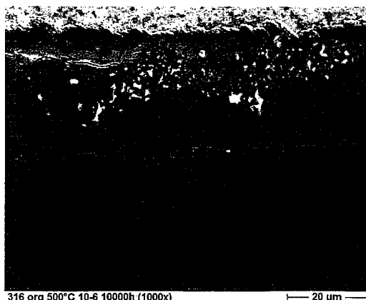
Fig. 2: Dissolution attack by grain boundary penetration in 316 FR after 10000 h of exposure at 500°C.
