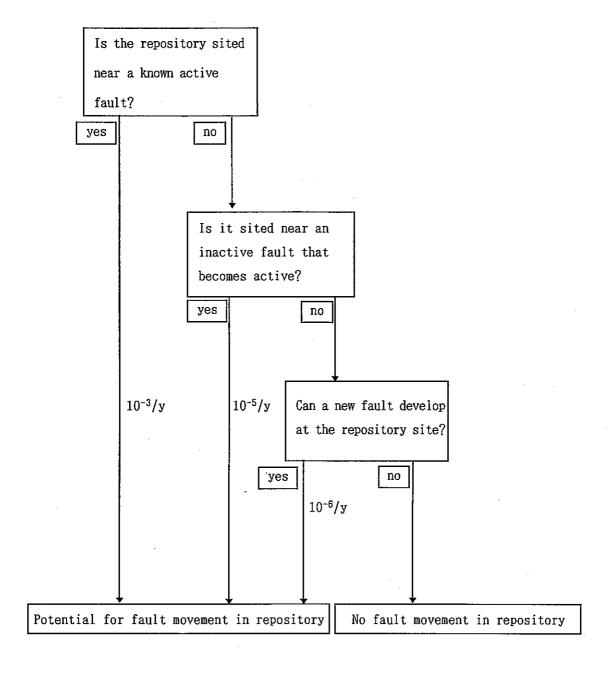
Figure 2 Logic Diagram Illustrating Conditions That Could Lead to Fault
