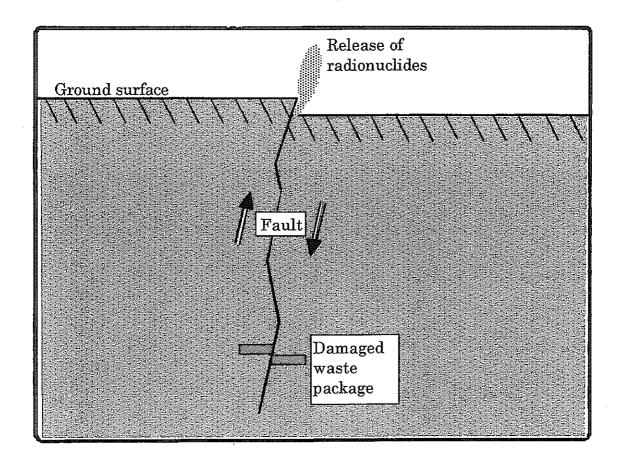
Figure 1 Schematic Diagram Depicting Postulated Active Fault Scenario
