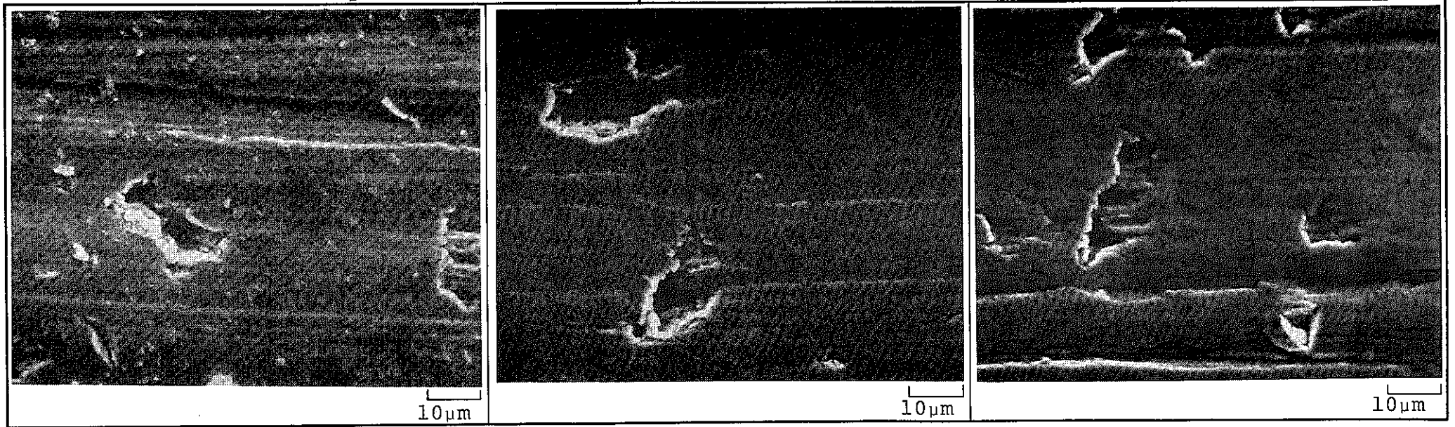
Fig. 5.47 Scanning Electromicrograph of Sliding Surface of Stator Side (400°C, 2m/s, 4.0kg/mm 2 , 240s)
