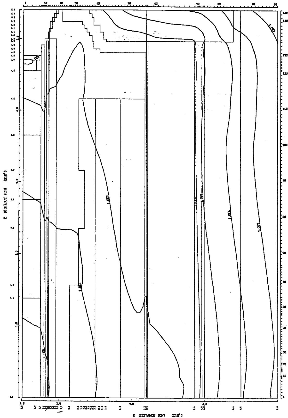
Fig. 2.4.28 Gamma-Ray Isodose Contours for Step 2 Calculation
