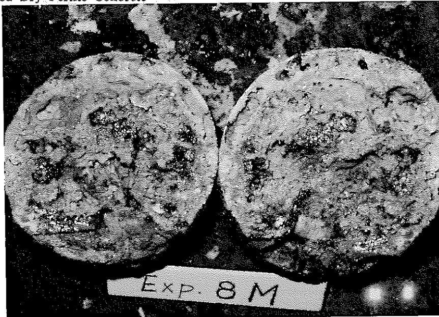
Photo.11 Cross Section of Reacted Perlite Concrete
