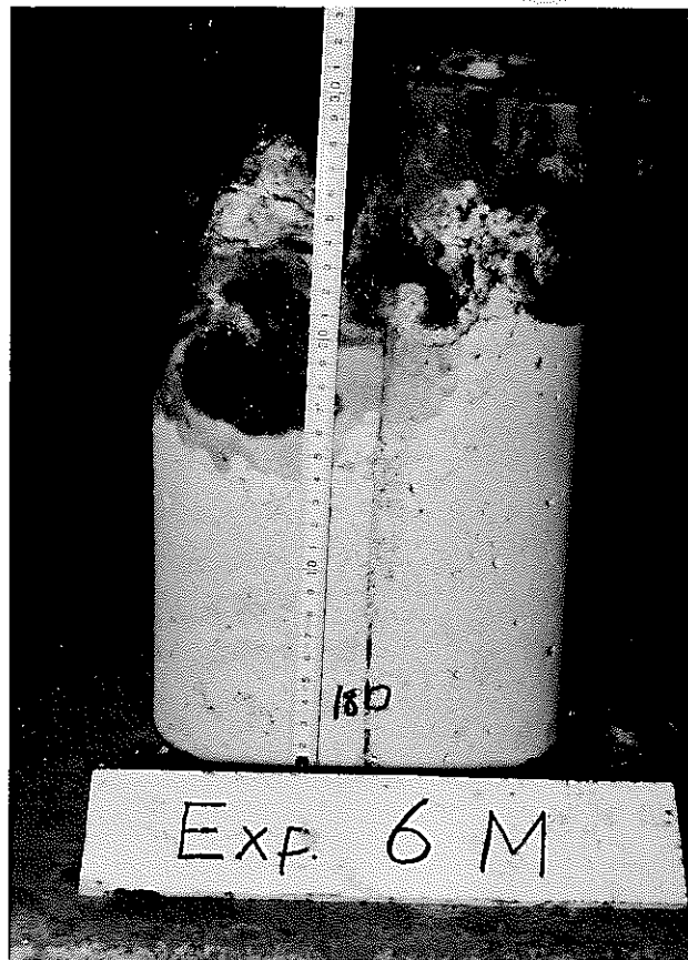
Photo. 8 Reacted Alumina Concrete at 530℃
