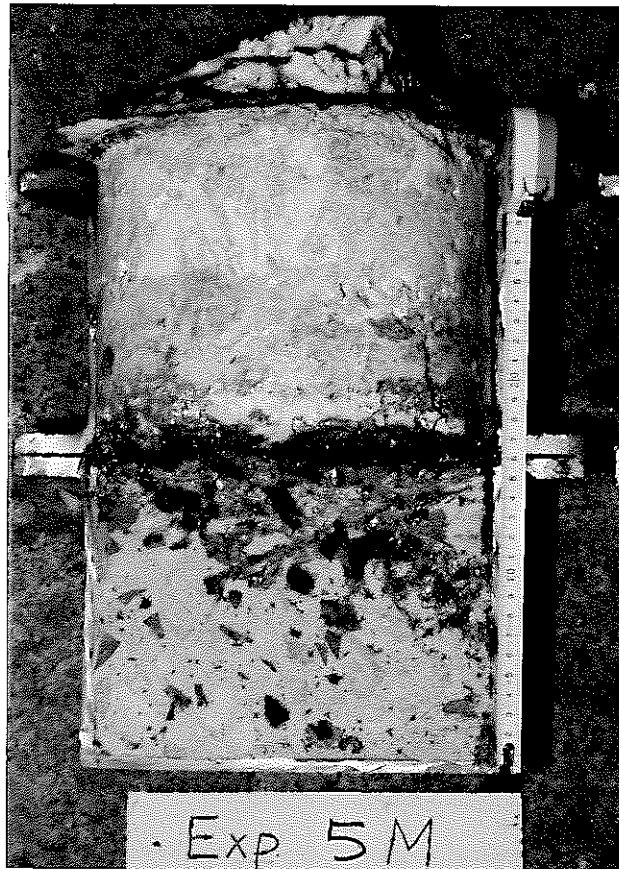
Photo. 7 Reacted Two Layer's Concrete (Perlite and Graywacke)
