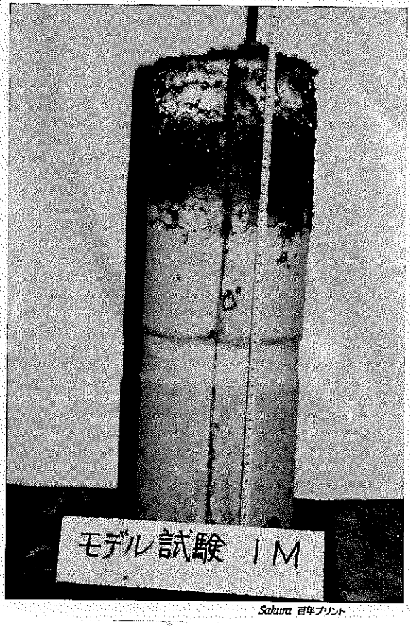
Photo 2. Reacted concrete ( Exp. 1M)
