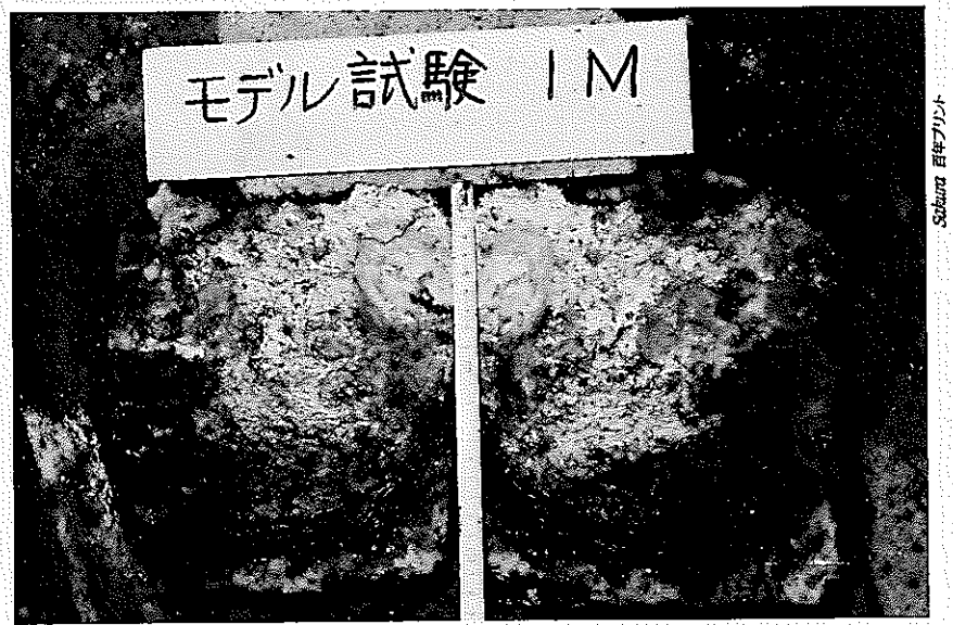
Photo 3. Vertical cross section of reacted concrete
