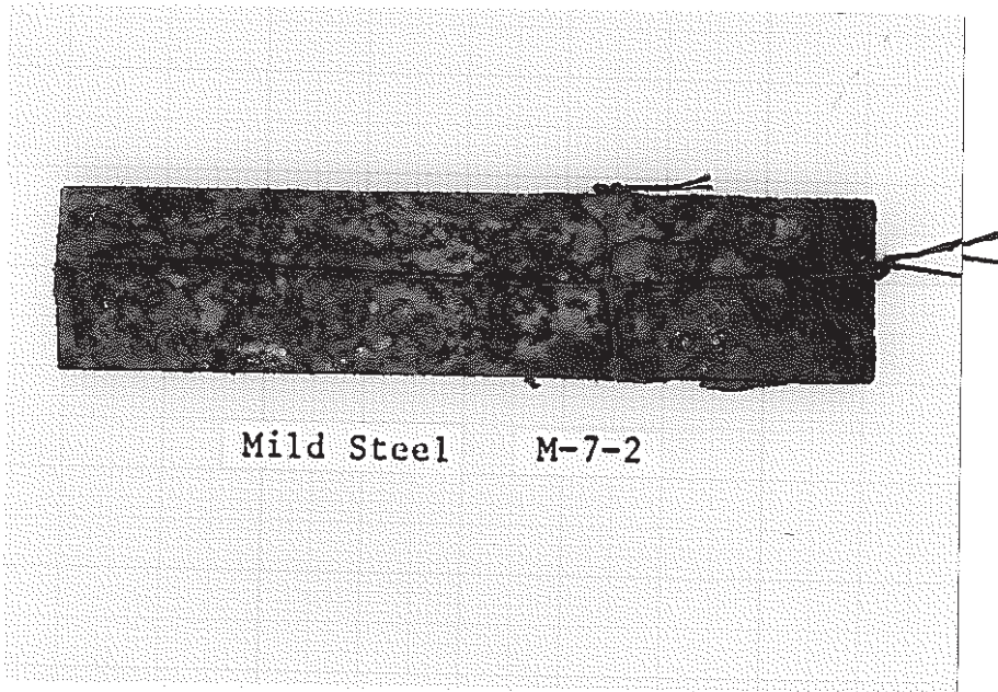
Photo 3—4(1) Mild Steel Test Sample after 1 Year Immersion Corrosion Test. 1年埋設後の軟鋼平板試験体
