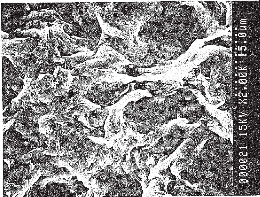
Photo. 2.3-39 SEM Picture of Dense Na-Bentonite. \times 2000 , 200 ~ 400 mesh, Sampled from the Surface, Drying without Freezing Mixture.
