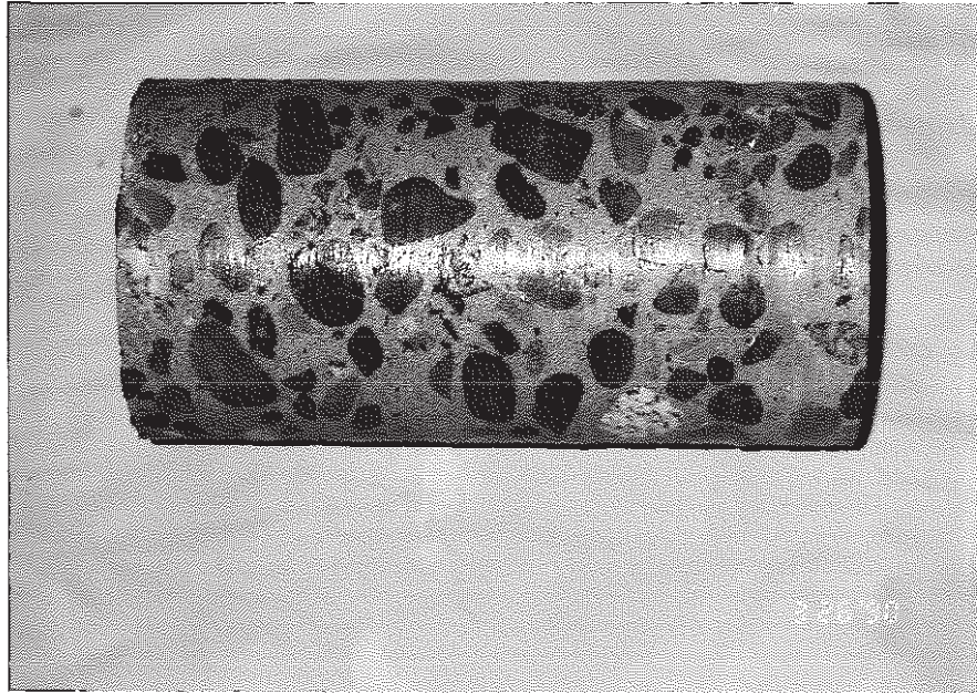
写真 - 20 透水試験用供試体 Photo. - 20 Core Sample of Permeability Test
