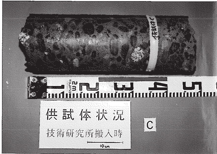
写真-17 内部コア側面 Photo.-17 Side Surface State of Core (Inside)
