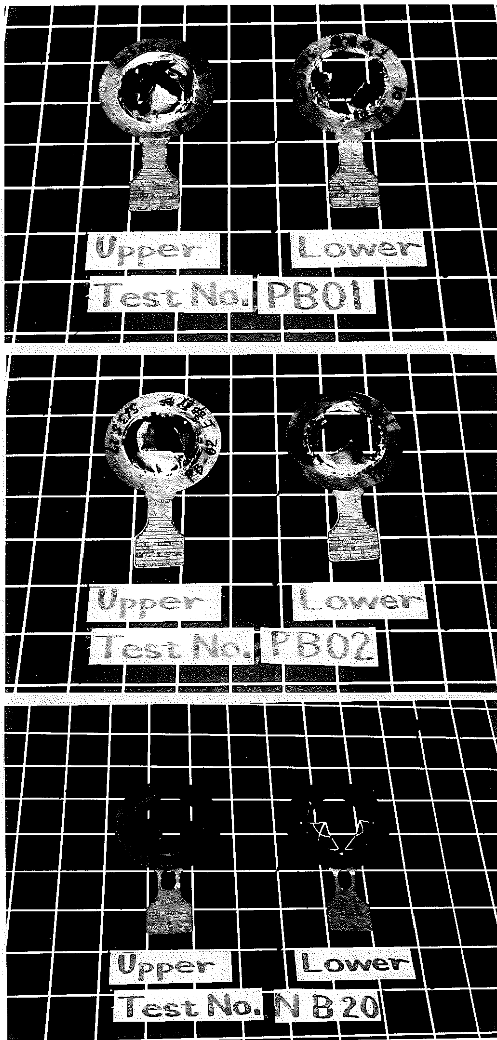
Photo 6.1 Appearance of Rupture Discs after Tests
