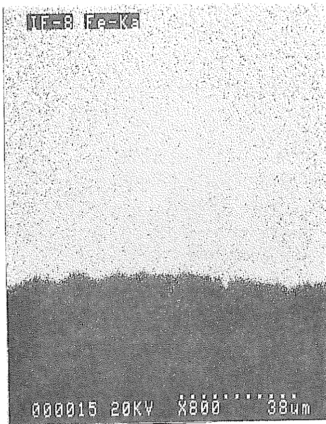
Figure 59 Scanning Electron Micrograph and Elemental Analysis by EPMA for IF-8 Cladding reacted with Iodine at 600°C. (IF-8 Specimen)
