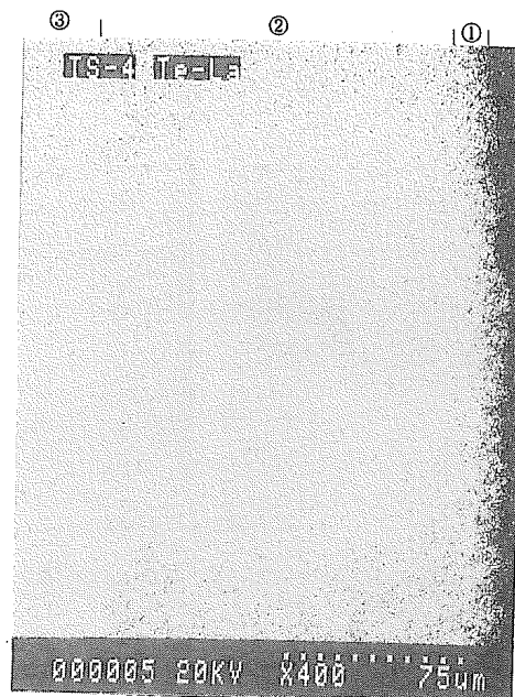
Figure 34 Scanning Electron Micrograph and Elemental Analysis by EPMA for Modified SUS316 Cladding reacted with Tellurium at 700°C. (TS-4 Specimen)
