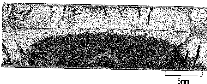
(b) fracture surface of fatigue (550°C, \Delta\delta=7.1\text{mm} )
