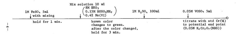
Figure 1. Determination of U content by a method similar to NBL-Davies-Gray method.
