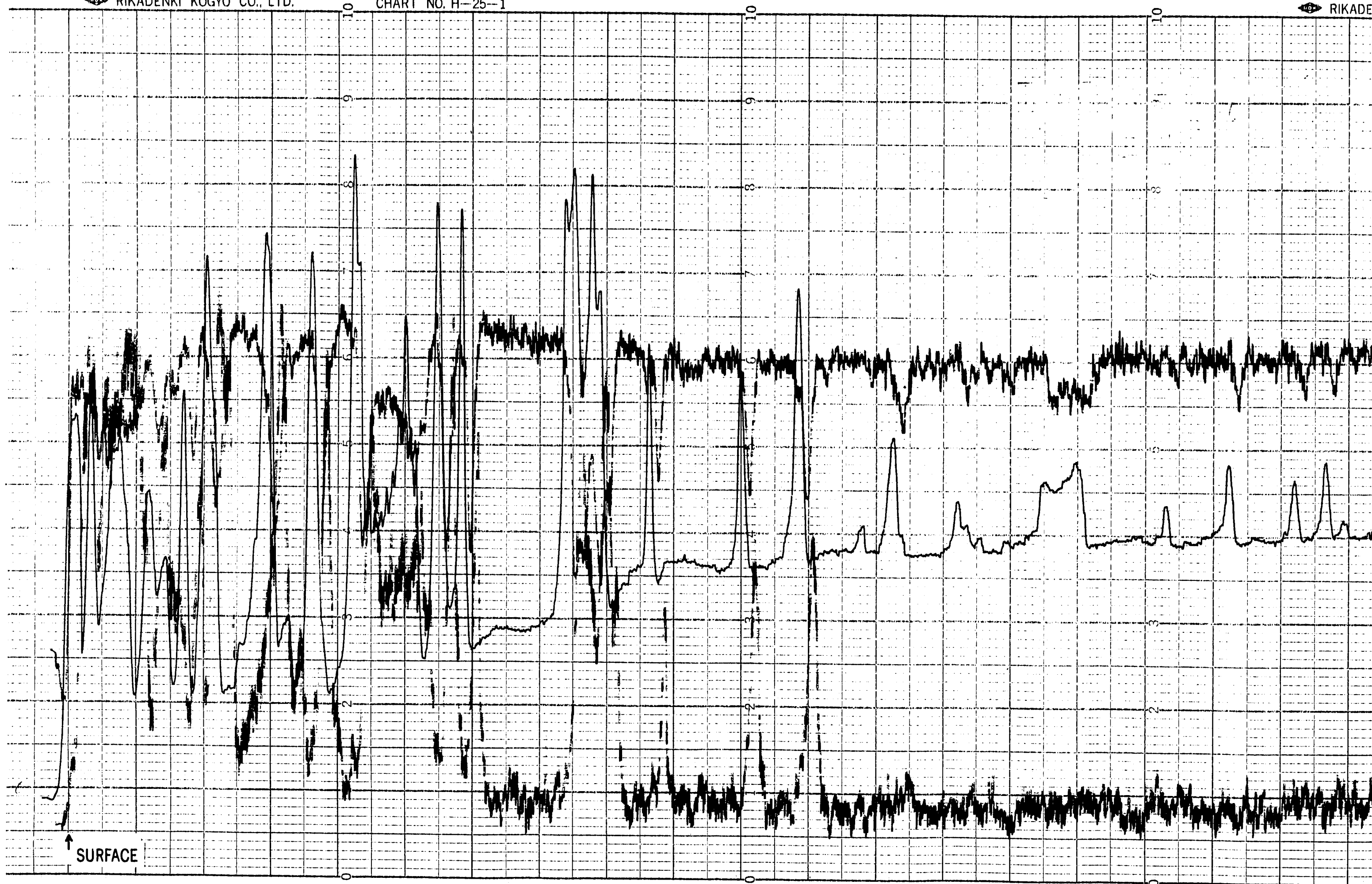
FIG. 7 XMA ANALYSIS OF SUS316 SPACER AFTER 850°CX500HR. HEATED, IN CONTACT WITH B_{3.5}C PELLETT.
