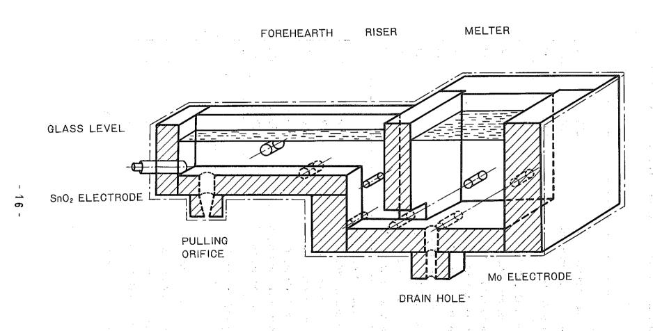
Fig. 1 Schematic of Joule Heated Ceramic Melter.
