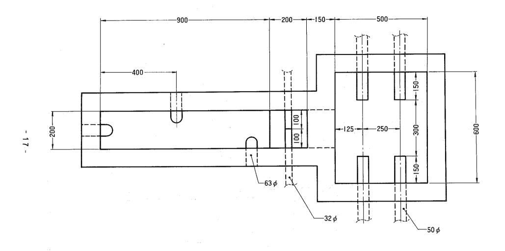
Fig. 2 Plane Figure of Engineering Scale Ceramic Melter.
