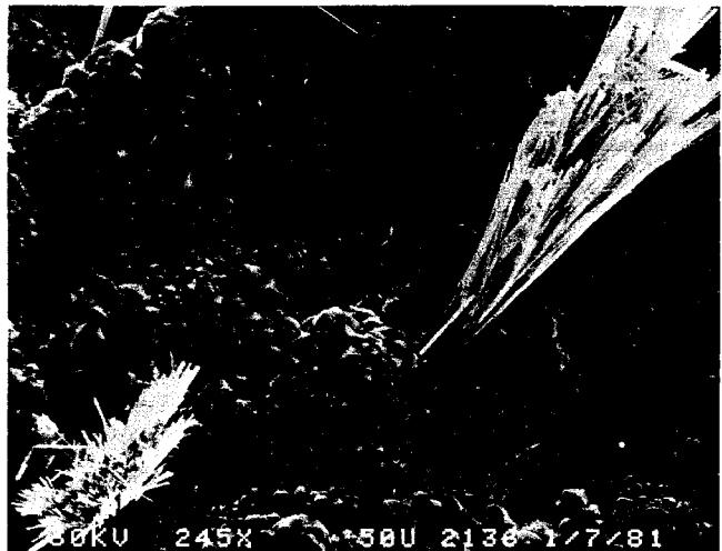
Photo. 3.20 A surface of supercalcine after hydrothermal treatment at 300°C and 30 MPa for 28 days.
