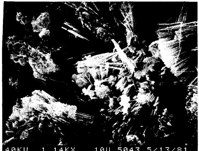
Photo. 3.33 Backfill materials altered by hydrothermal treatment with sintered ceramic at 300°C and 30 MPa for 28 days.
