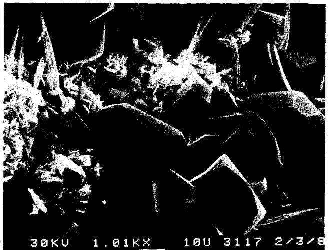
Photo. 3.15 A surface of sintered ceramic shard after hydrothermal treatment at 300°C and 30 MPa for 28 days.
