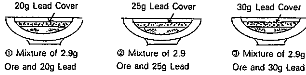
Figure 12-21 Scorfication assay, third step: combining ore and lead and covering with lead
