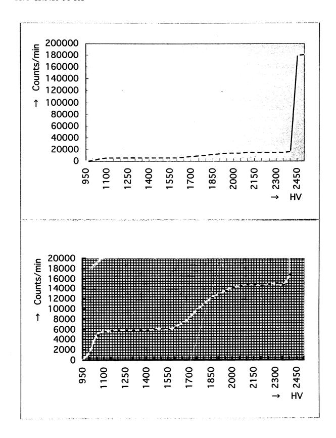
Figure 2  $\alpha$  and  $\beta$  plateaus of  $2\pi$  gas flow counter.
