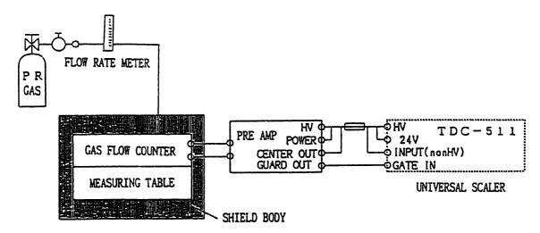
Figure 1 Block diagram of counting system.
