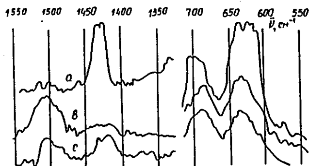
Fig. 5. Raman spectra in the areas 1550-1350\text{ cm}^{-1} and 750-550\text{ cm}^{-1} for Comp.C: a) before ageing and after one-month ageing, b) of the irradiated surface and c) of the nonirradiated surface.
