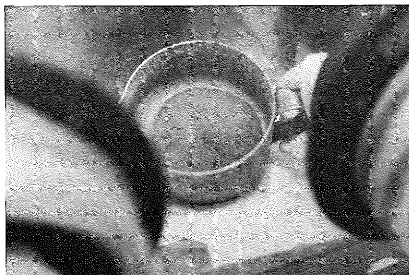
Photo. 4-6 Recovered Mixed Oxide (MOx) and Uranium 回収MOx粉末及び回収U粉末
