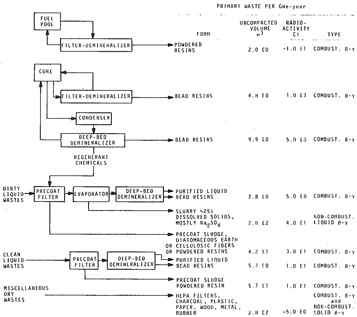
FIGURE 2.7. Sources and Characteristics of Non-Gaseous Wastes from 1-GWe BWR with Deep-Bed Condensate Cleanup
