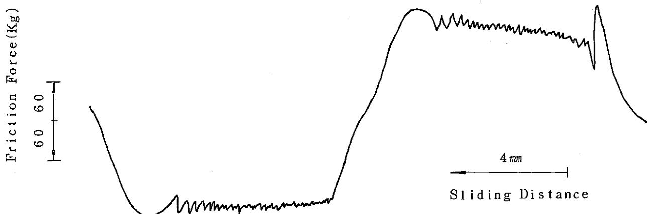
Friction Diagram at Test under 200Kg Load after Dwell Time (1000mm)
