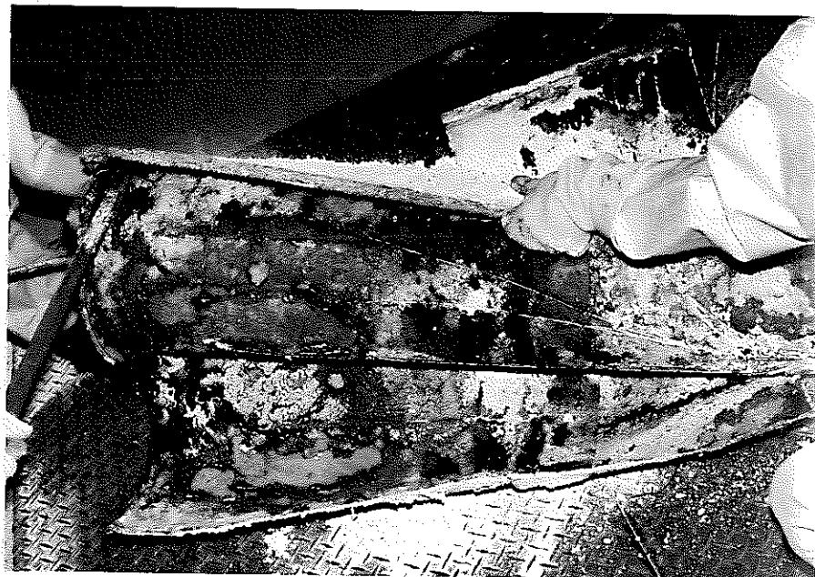
Photo. 3 : Disassembling of Simulated Sodium Pipe after the Test
