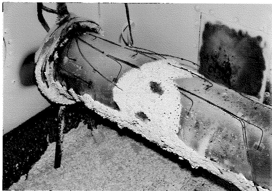
Photo. 2 : Simulated Sodium Pipe and Floor Liner in Combustion
