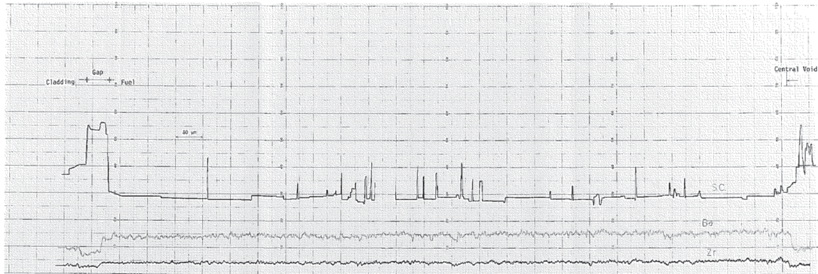
Chart 2 Line Analyses by Zr-La and Ba-La from the Fuel Center to Cladding (Specimen No.70A644)
