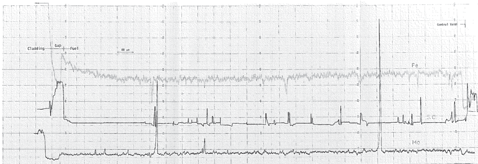
Chart 5 Line Analyses by Fe-K \alpha and Mo-L \alpha from the Fuel Center to Cladding (Specimen No.70A644)
