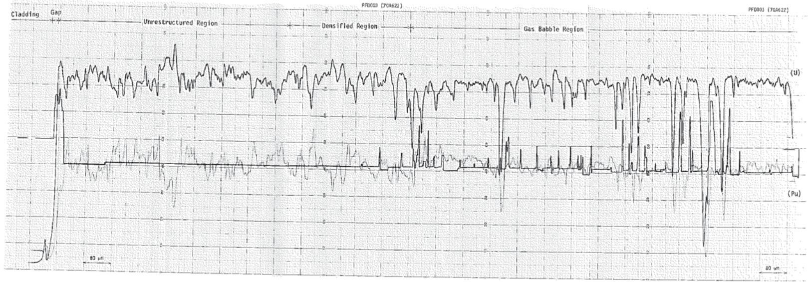
Chart 9 Line Analyses by U-M \alpha and Pu-M \beta from the Fuel Center to Cladding (Specimen No.70A662)
