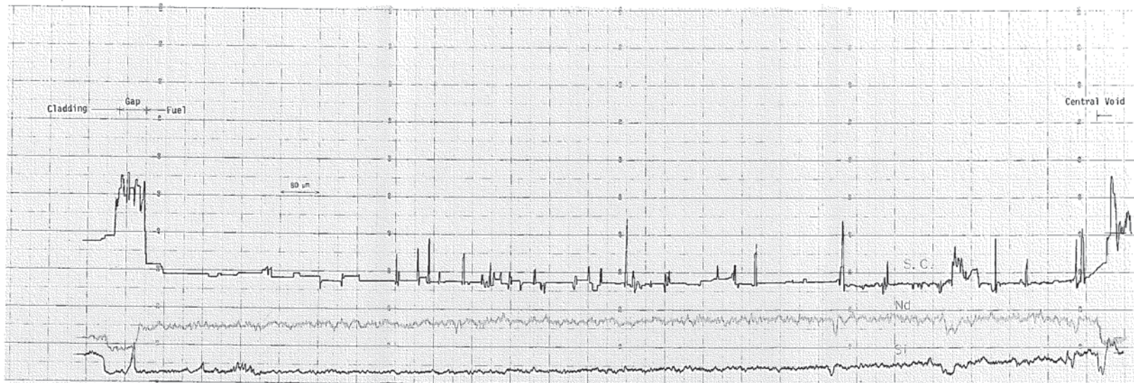
Chart 4 Line Analyses by Si-K \alpha and Nd-L \alpha from the Fuel Center to Cladding (Specimen No.70A644)
