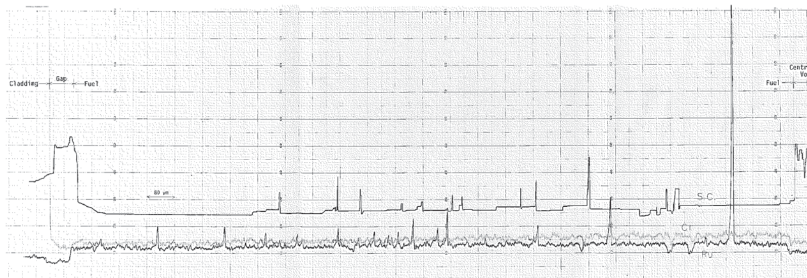
Chart 6 Line Analyses by Ru-L \alpha and Cr-K \alpha from the Fuel Center to Cladding (Specimen No.70A644)
