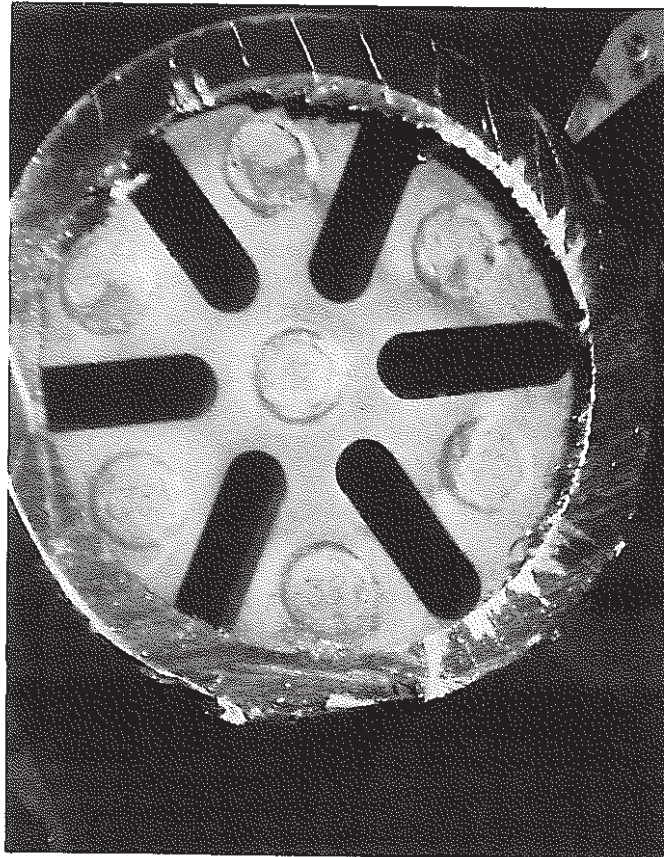
Photo 19 Holding Condition of Absorber Pin in Lower Grid Plate ( MCR006 )
