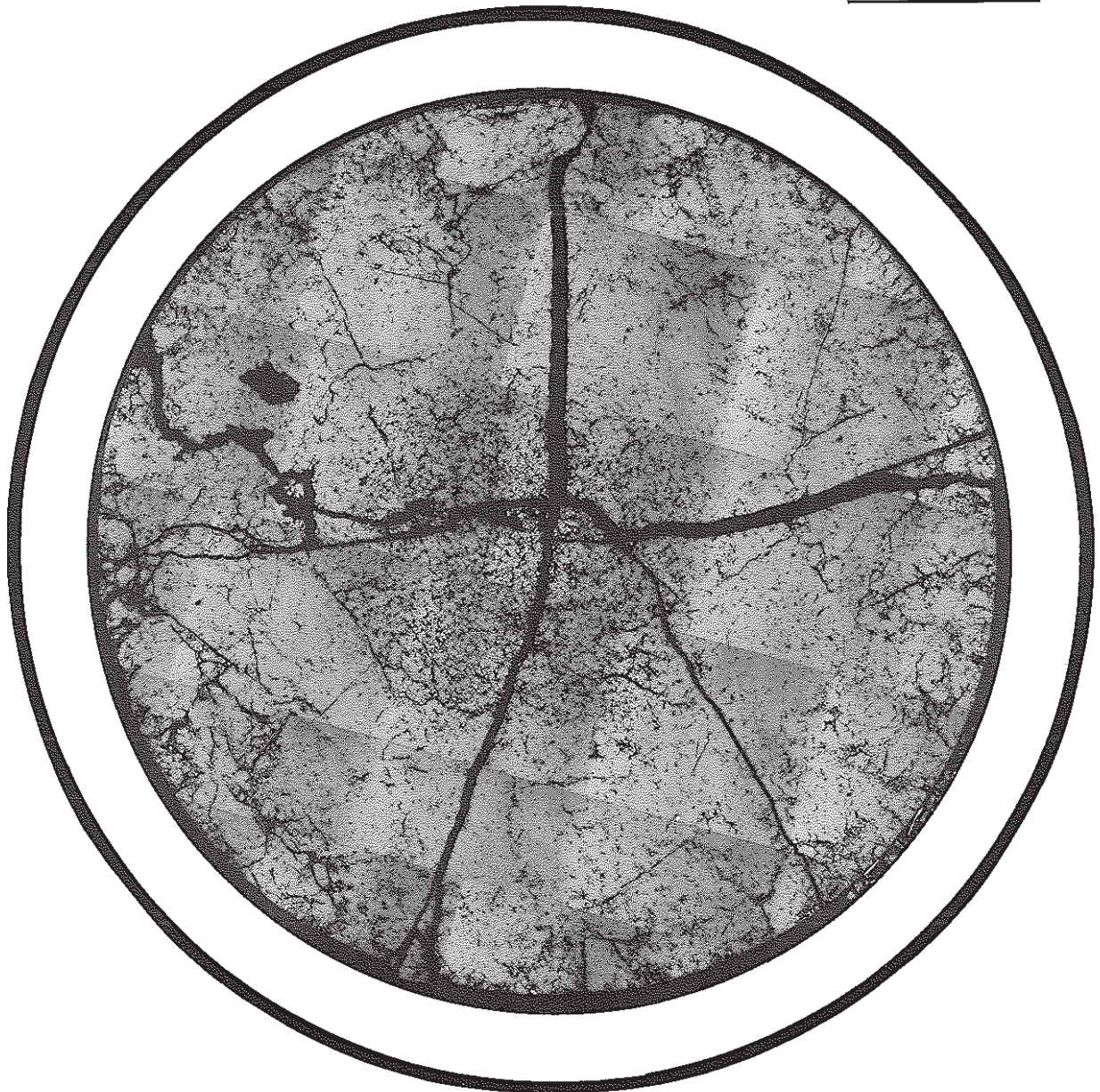
Photo 3 Ceramography of JOYO MK-II core fuel (636423 sample, as polished)
