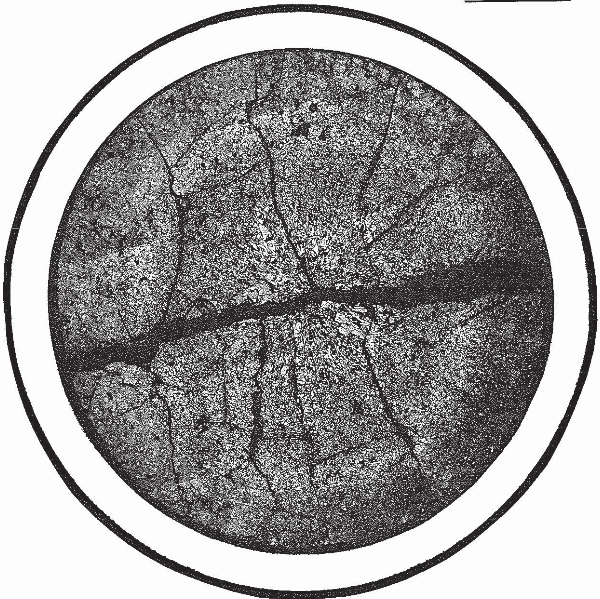
Photo 15 Postirradiation ceramography of JOYO MK-II core fuel (661322 sample, etched)
