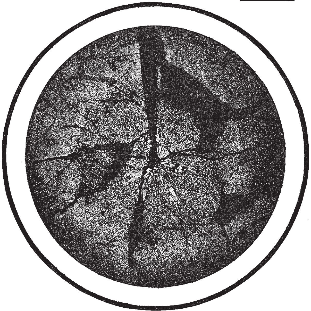
Photo 7 Postirradiation ceramography of JOYO MK-II core fuel ( 660222 sample, etched )
