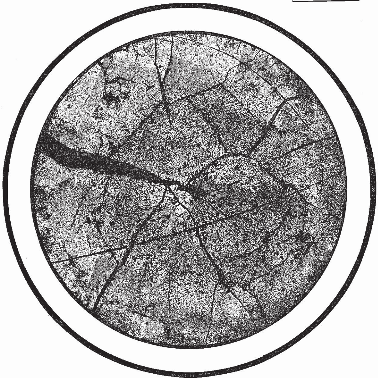
Photo 10 Postirradiation ceramography of JOYO MK-II core fuel (660522 sample, as polished)
