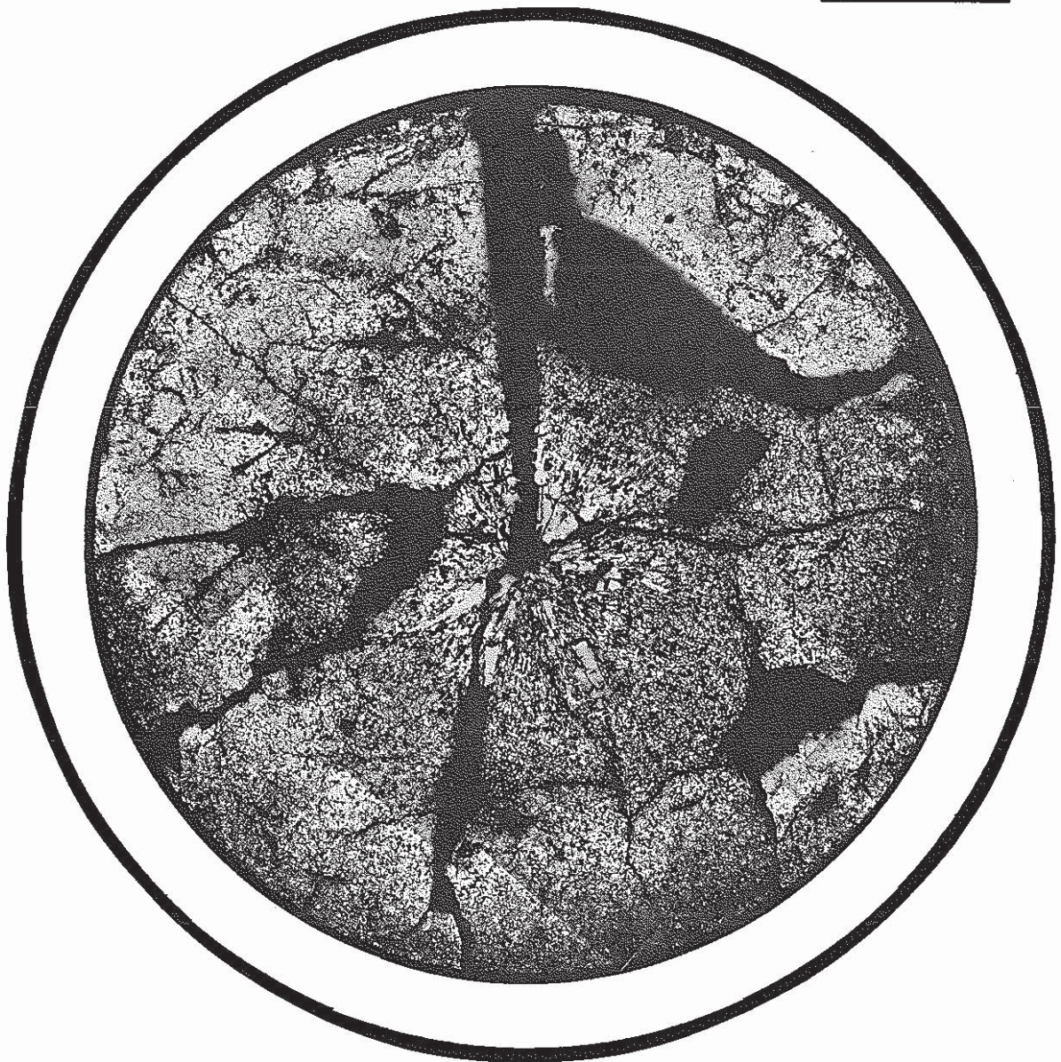
Photo 6 Postirradiation ceramography of JOYO MK-II core fuel ( 660222 sample, as polished )
