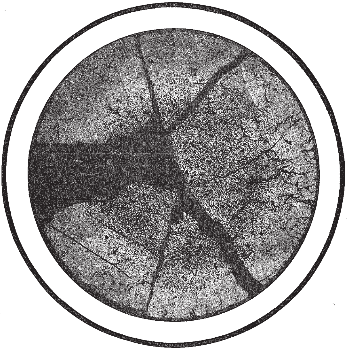
Photo 23 Postirradiation ceramography of JOYO MK-II core fuel (661362 sample, etched)
