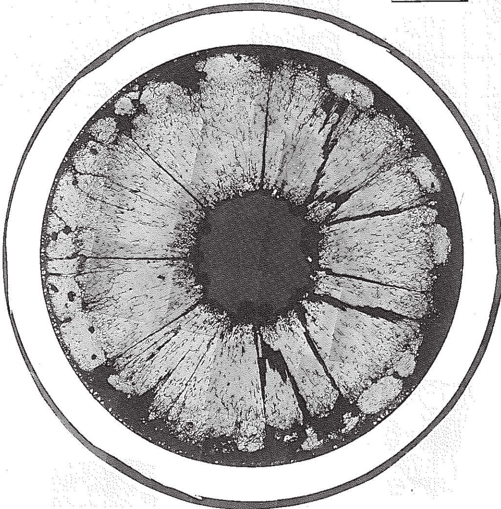
Photo 8 Postirradiation ceramography of Rapsodie core fuel (Sample XC04A1)
