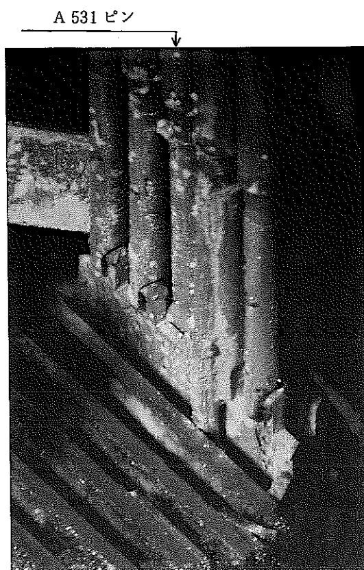
Photo. 10 Condition of a pin Comming off the Knock-Bar
