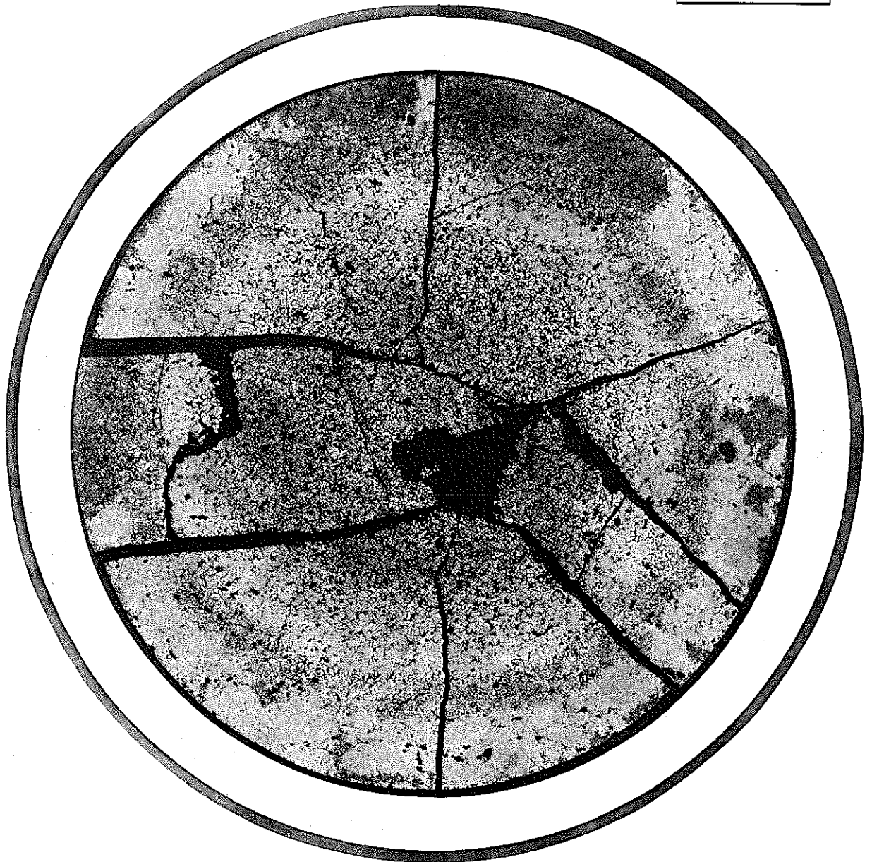
Photo. 10 Postirradiation ceramograph of the transverse section of JOYO MK-1U core fuel (7064A3 sample)
