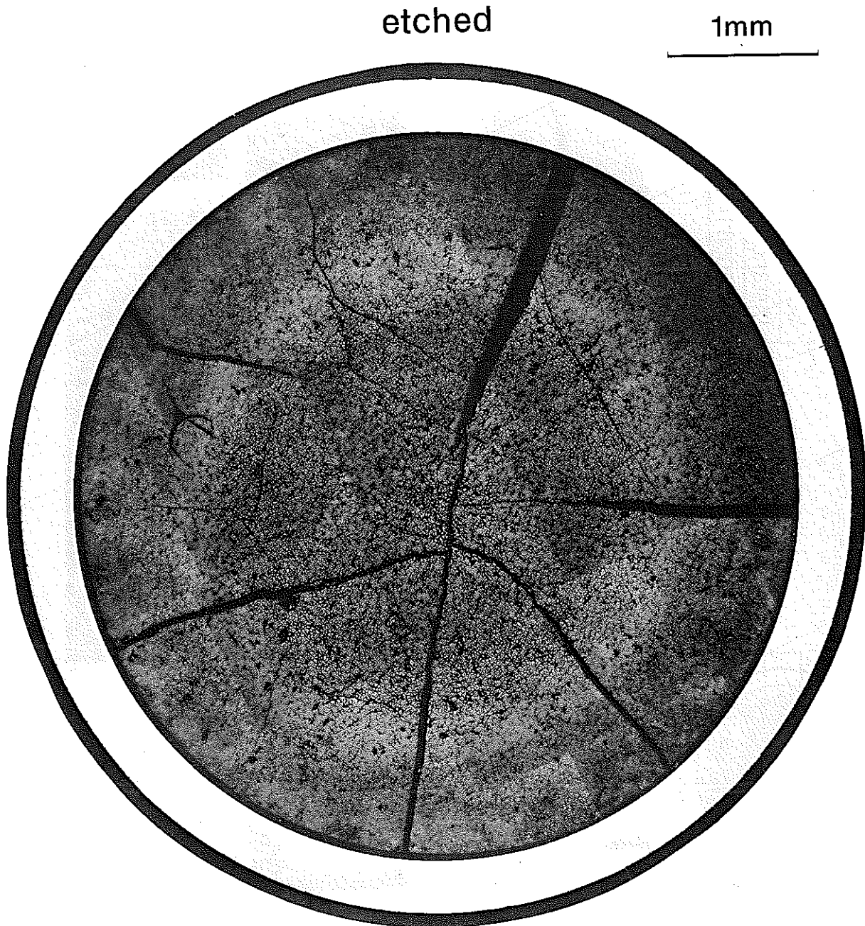
Photo. 5 Postirradiation ceramograph of the transverse section of JOYO MK-II core fuel (706442 sample)
