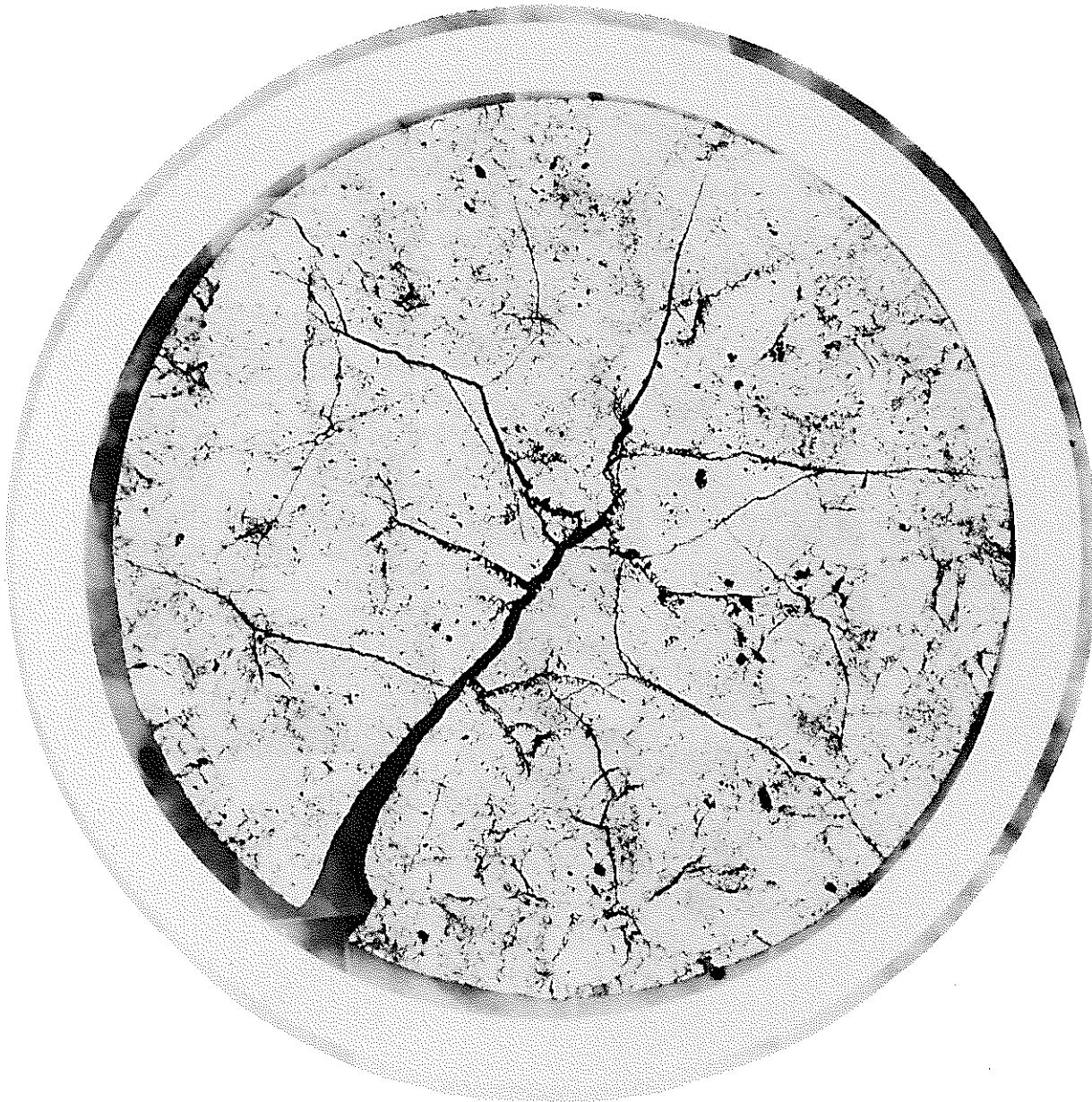
Photo.7 Optical micrograph of the transverse section of the core fuel pin ( specimen No. A 60922 ) as polished
