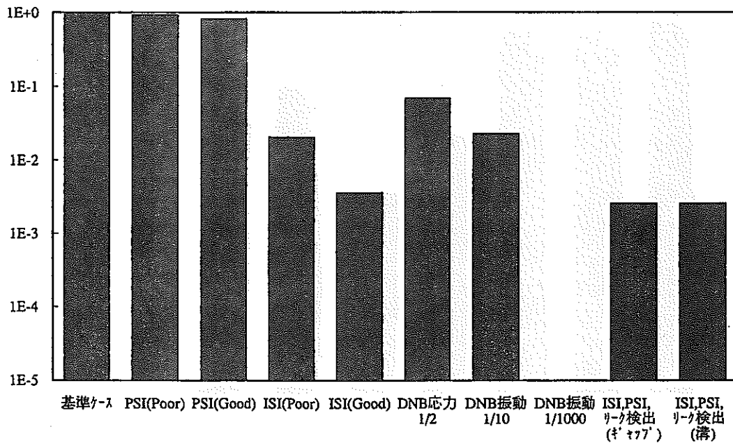
Fig.2.2-17 Influence of various parameters on cumulative probability of break (Inner tube : Axial crack)
