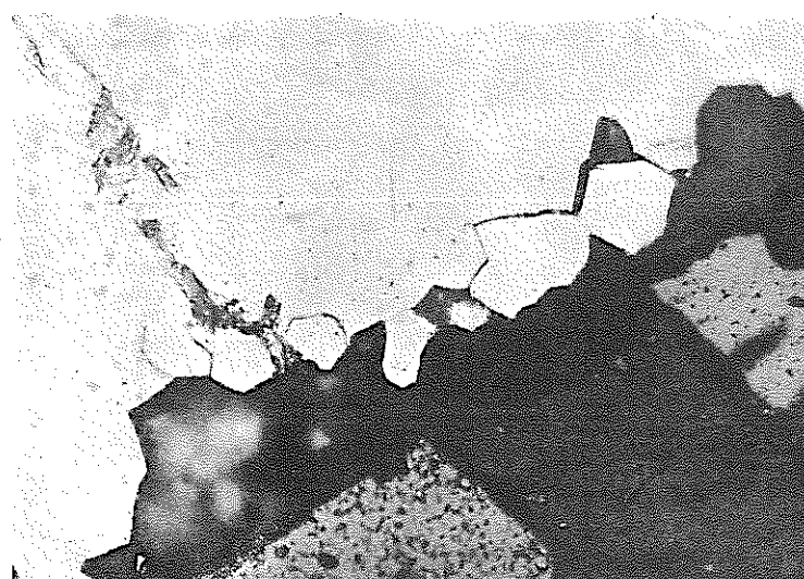
Photograph 23. Damage to inner surface of cladding tube Pin-E-20502
