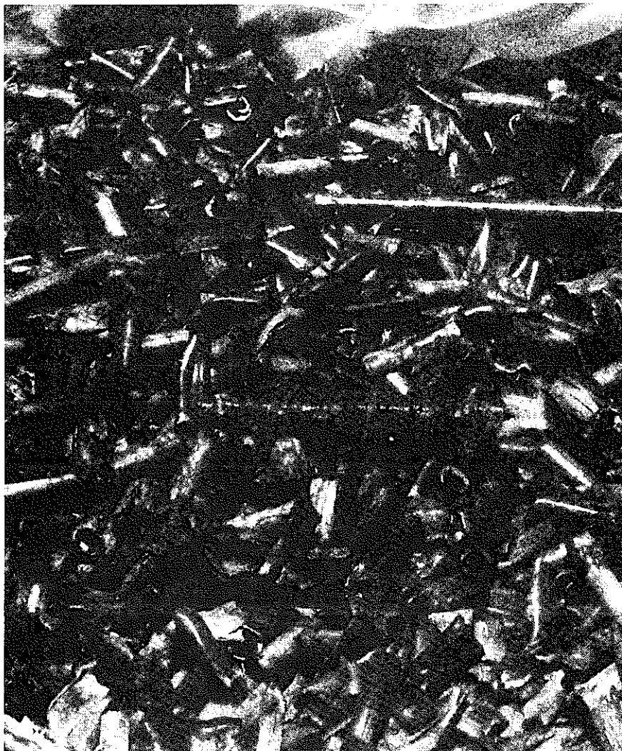
FIG. 2. Zircaloy cladding scraps from fuel dissolution at Cogéma plant, La Hague, France.
