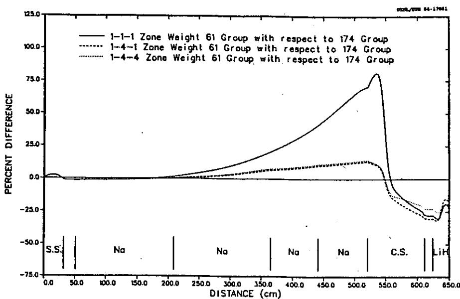
Fig. 13. Comparison of 4-in. Bonner ball responses calculated using fine-group cross sections and 61-group neutron cross sections collapsed using three different zone-averaged weighting functions.
