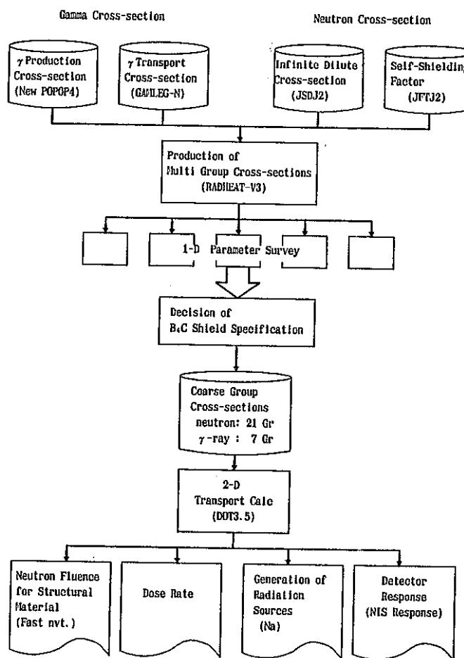
Fig. 2. Schematic Flow Diagram of Shielding Design
