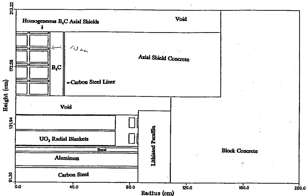
Fig. 2. Axial Shield Experiment 2-D Calculational Geometry Model for Case 2.
