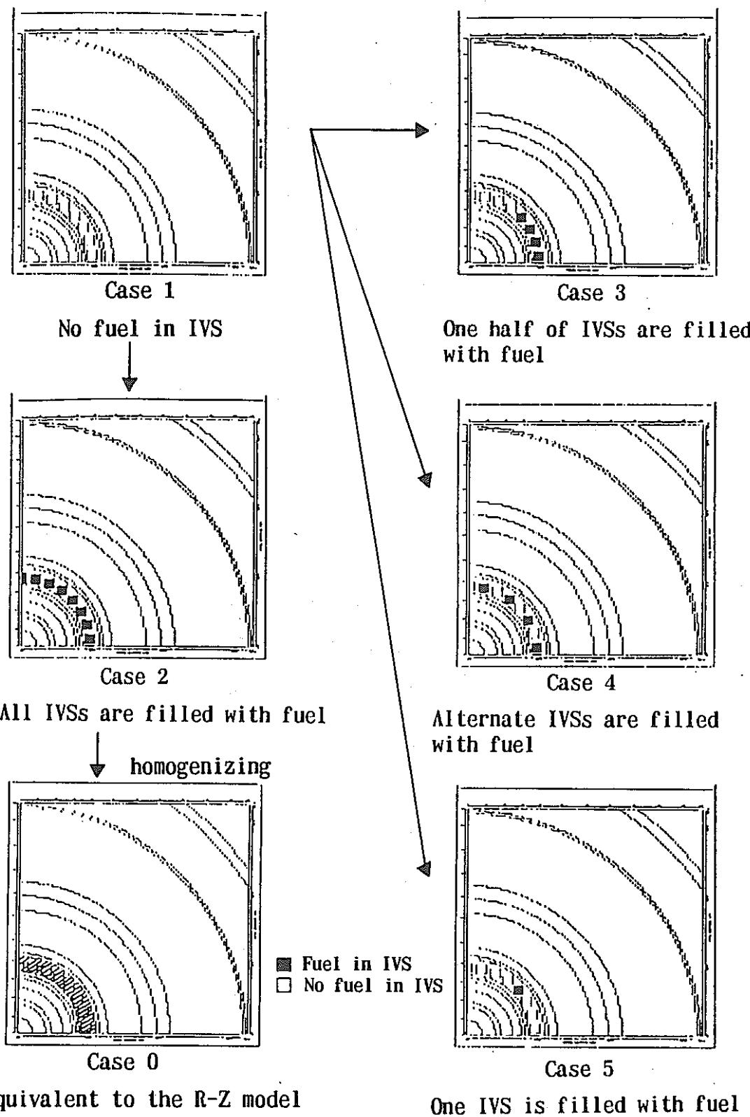
Fig.8 Models for the 2D X-Y calculations by DOT3.5
