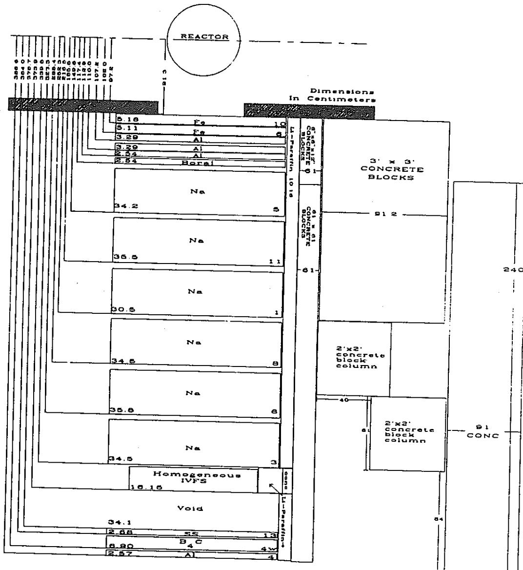
Figure 51. Schematic of SM-2 plus shield configuration for Item IIIF.
