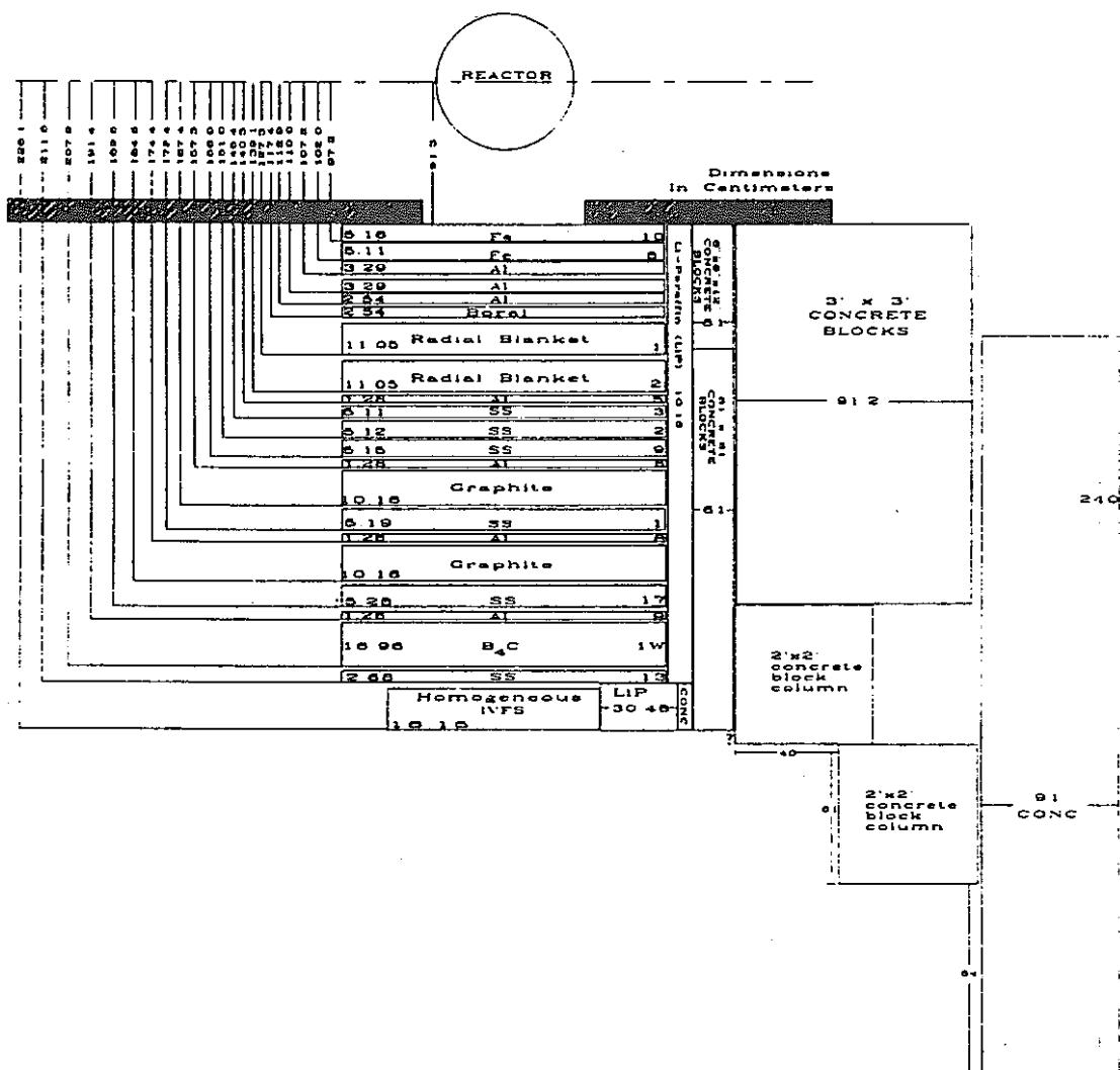
Figure 35. Schematic of SM-1 plus shield configuration for Item IIK.
