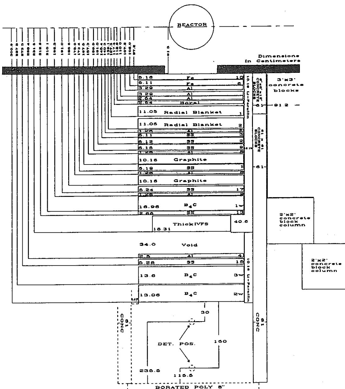
Figure 44B. Schematic of SM-1 plus shield configuration for Item IIP (Note: This mockup was used for measurements behind B<sub>4</sub>C slab 2W only).
