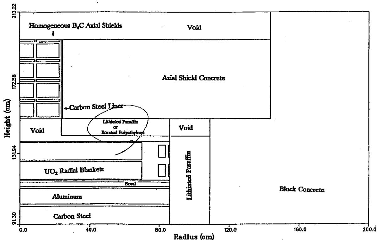
Fig. 4. Axial Shield Experiment 2-D Calculational Geometry Model for Cases 4 and 5.
