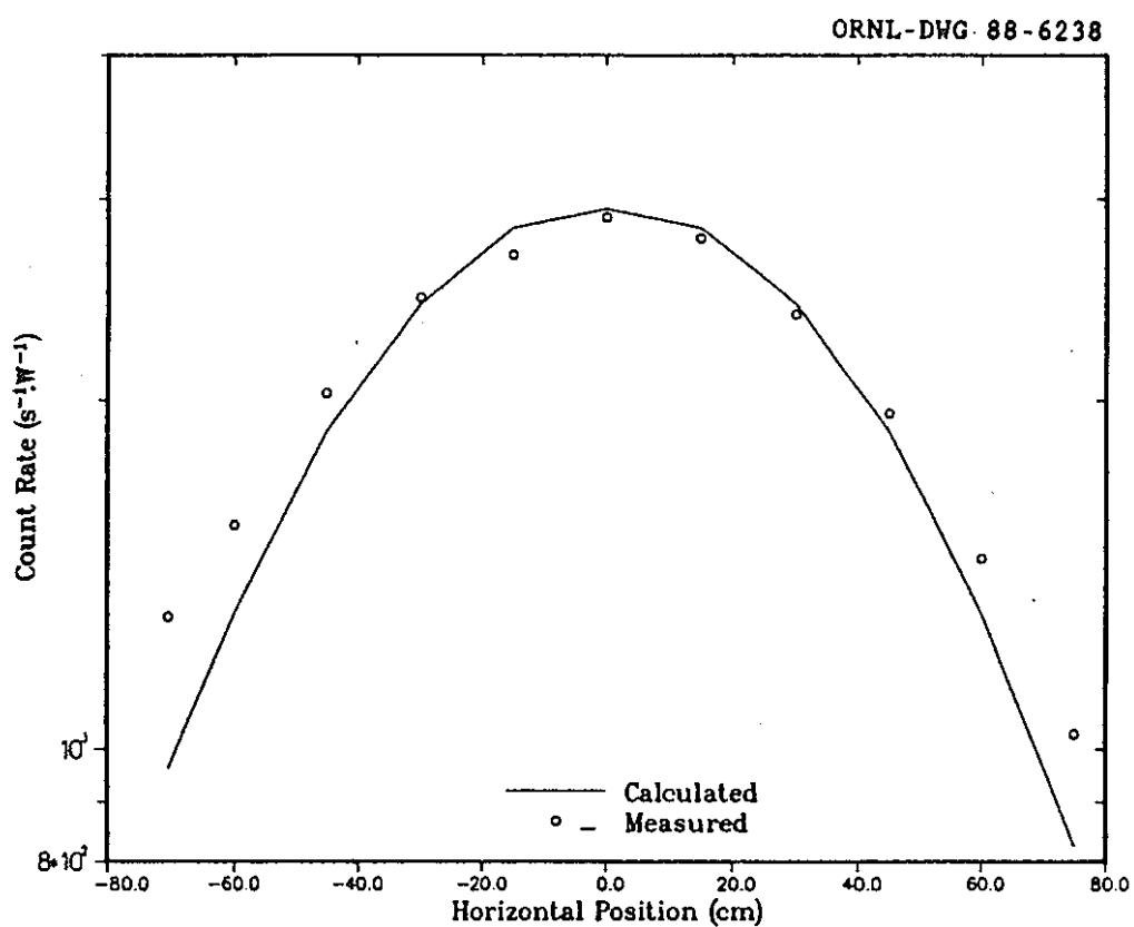
Figure 9. Comparison of calculated and measured 5-in. Bonner ball count rates for a horizontal traverse 30 cm behind Configuration I.A (C/E range: 0.74-1.06).
