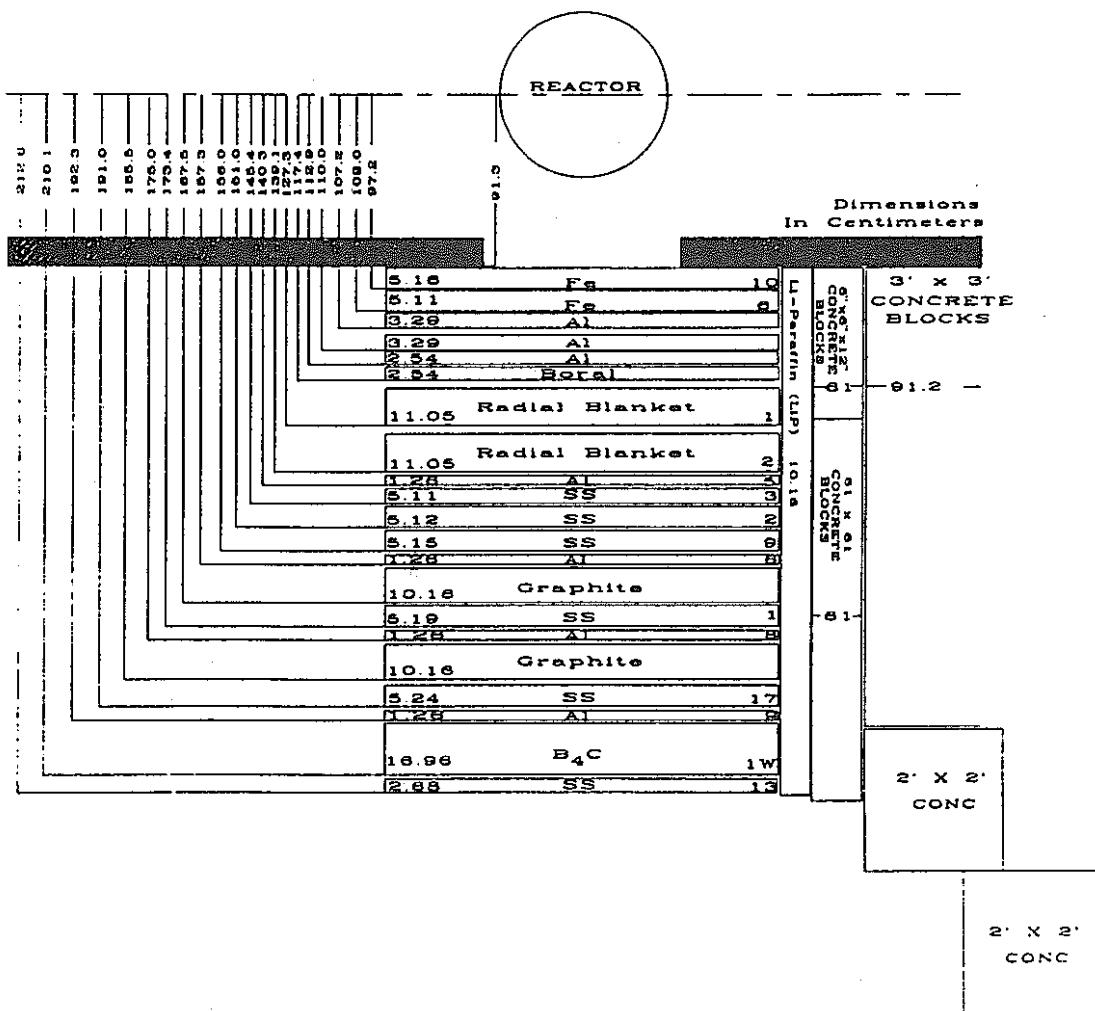
Figure 32. Schematic of SM-1 plus shield configuration for Item IIIH.
