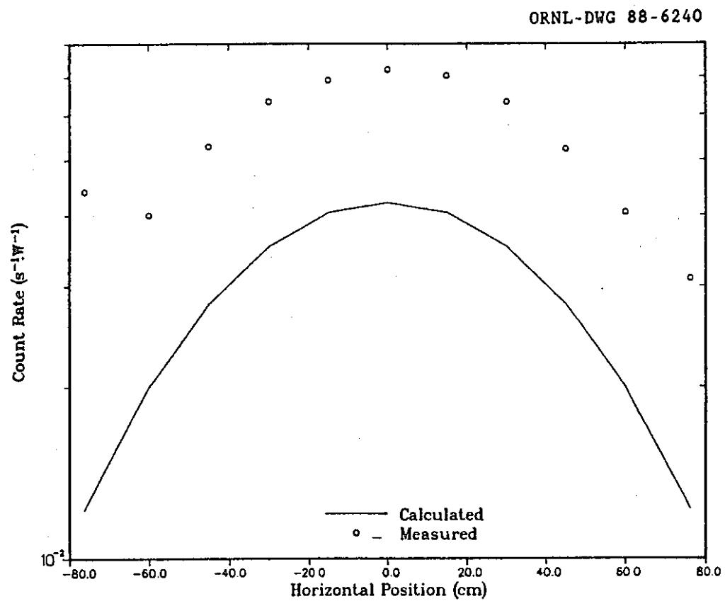
Figure 11. Comparison of calculated and measured 5-in. Bonner ball count rates for a horizontal traverse 30 cm behind Configuration II.D (C/E range: 0.28-0.58).
