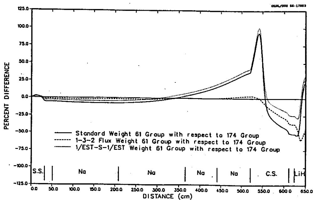
Fig. 15. Comparison of 4-in. Bonner ball responses calculated using fine-group cross sections and 61-group neutron cross sections collapsed using three final weighting functions.
