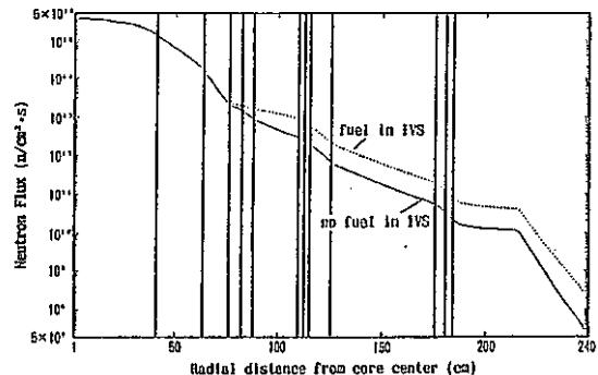
Fig. 7. Radial traverse of fast neutron flux
