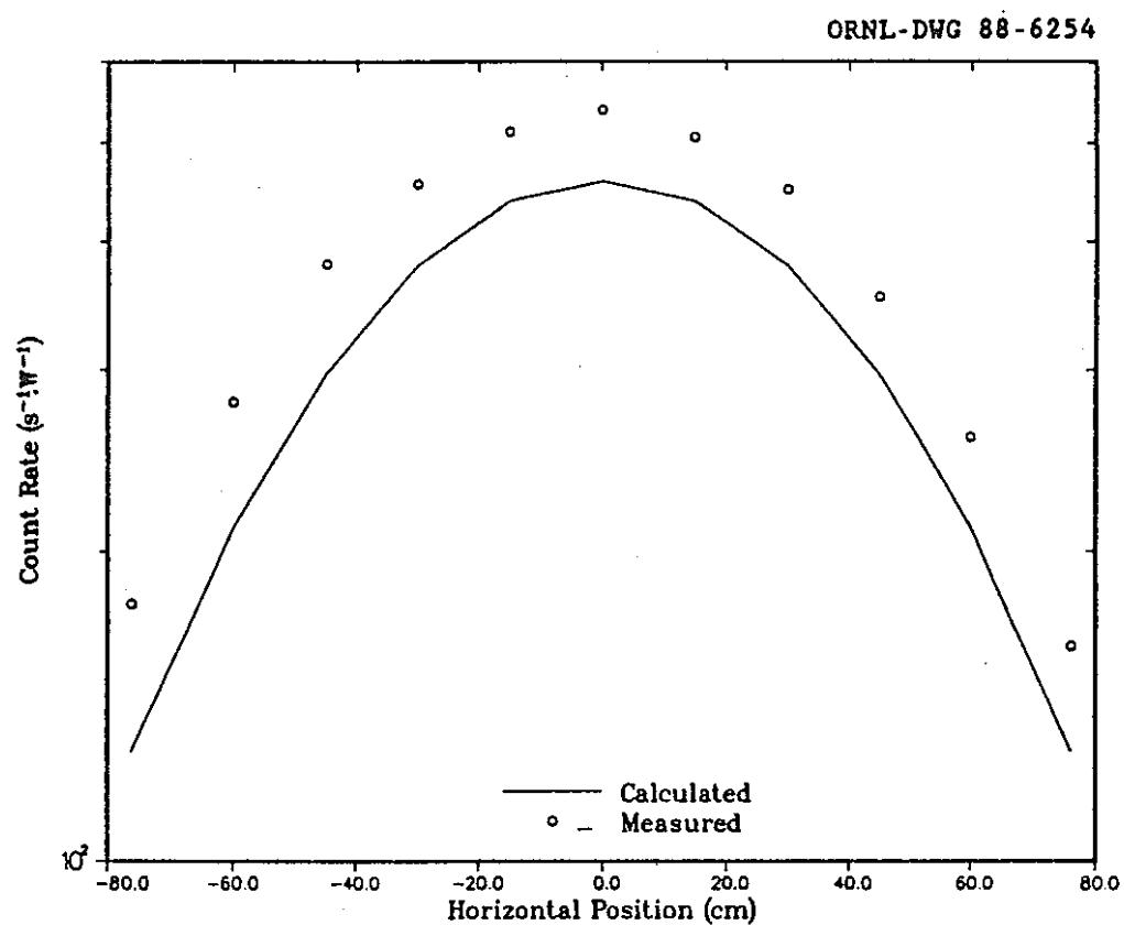
Figure 25. Comparison of calculated and measured 5-in. Bonner ball count rates for a horizontal traverse 30 cm behind Configuration VI.A (C/E range: 0.72-0.87).
