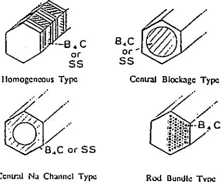
Fig. 2 Experimental Assembly of the Axial Shield Experiment
