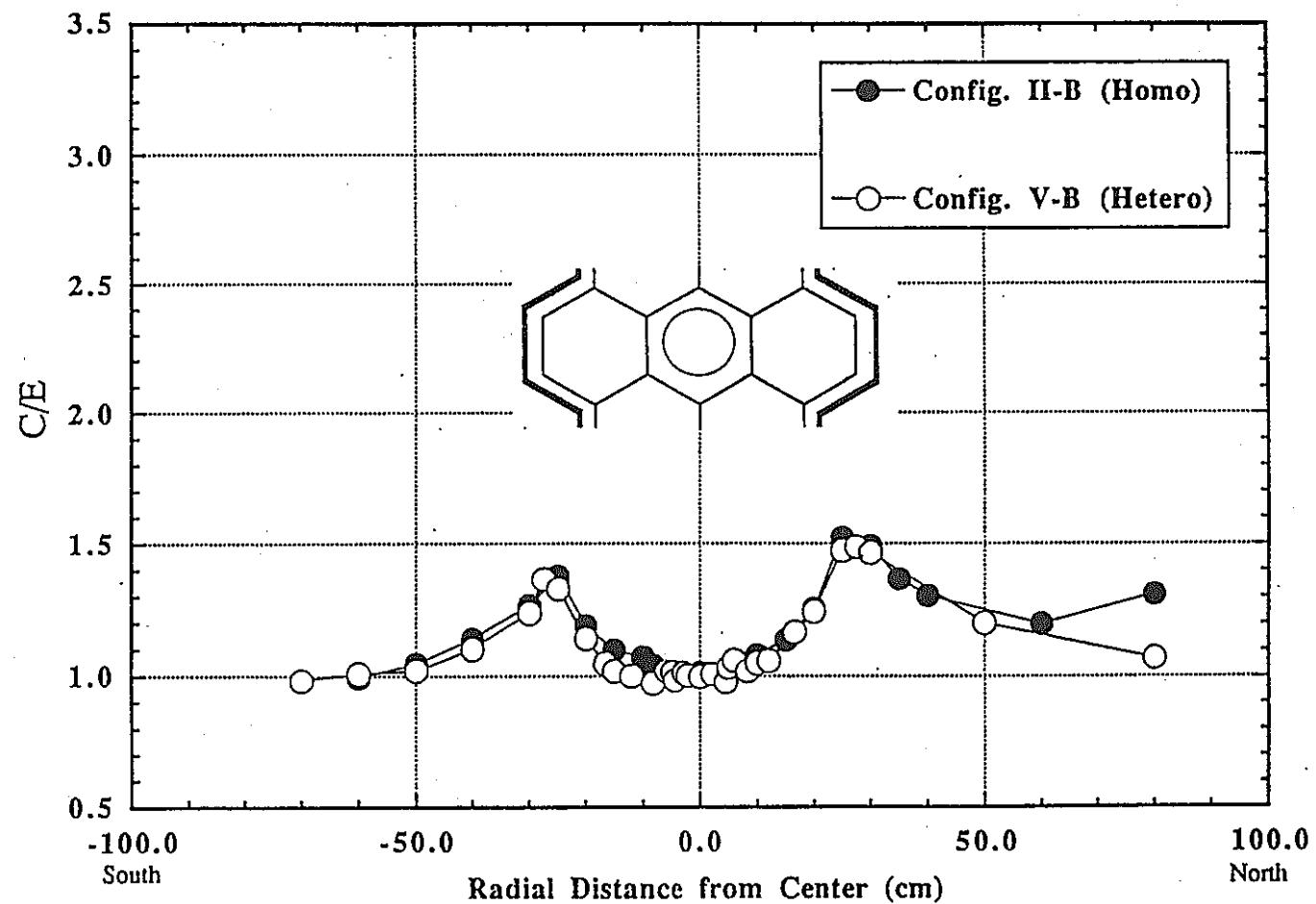
C/E Distributions of Hornyak Button Response for SS Type Axial Shield Configurations
