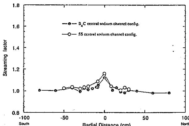
Fig. 3 Radial distribution of streaming factor derived from measured Hornyak button data.
