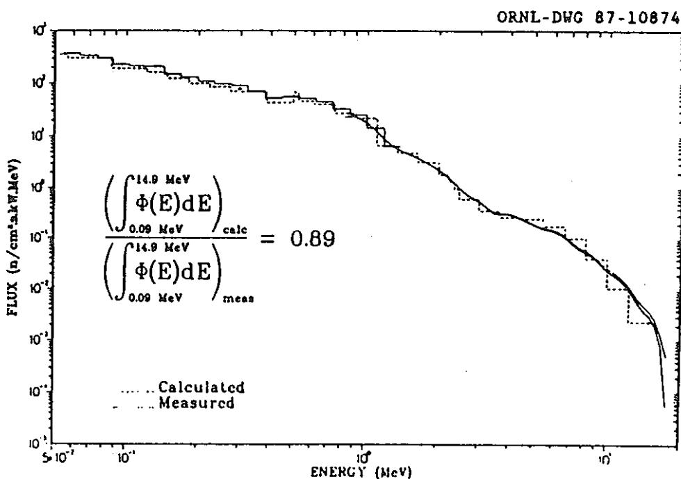
Fig. 5. Calculated versus measured  $E > 0.05$  MeV neutron spectra on centerline 42.8 cm behind Configuration IV.C.
