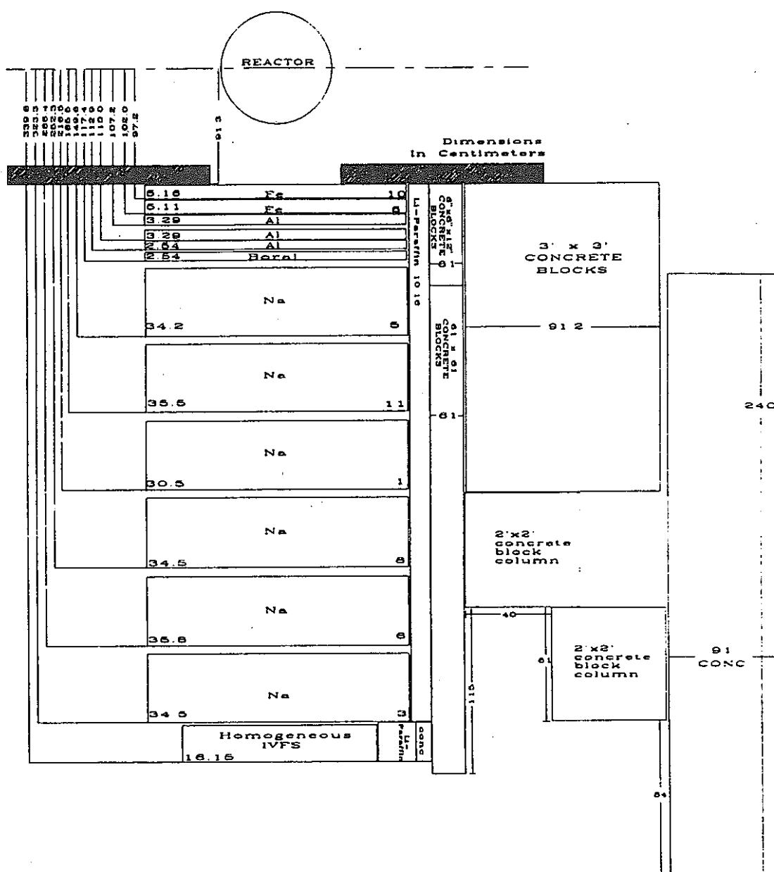
Figure 47. Schematic of SM-2 plus shield configuration for Item IIIB.
