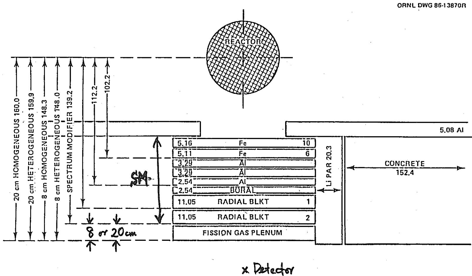
Fig. Schematic of Spectrum Modifier And Fission Gas Plenum Mockup
