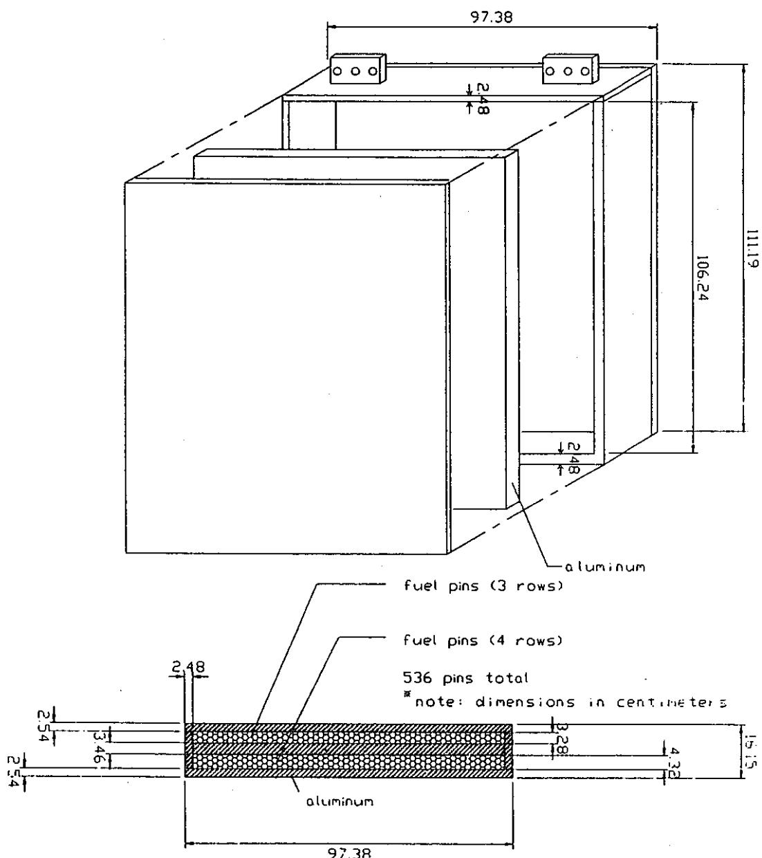
Figure 10. Schematic of homogeneous IVFS mockup (slab #3).
