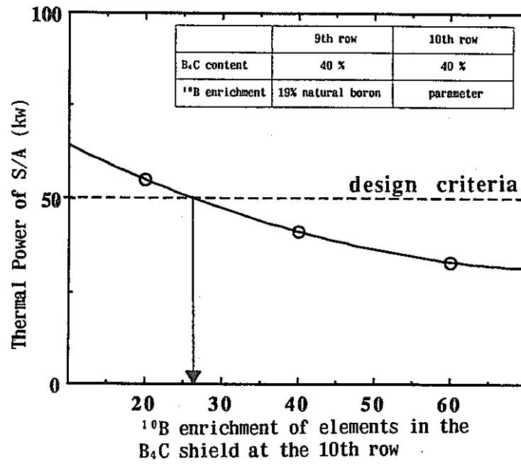
Fig. 4. Relationship between the thermal power of S/A in IVS and the <sup>10</sup>B enrichment of B<sub>4</sub>C element
