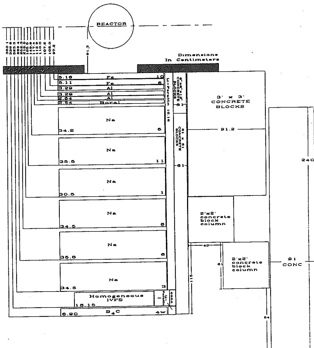
Figure 49. Schematic of SM-2 plus shield configuration for Item IID.
