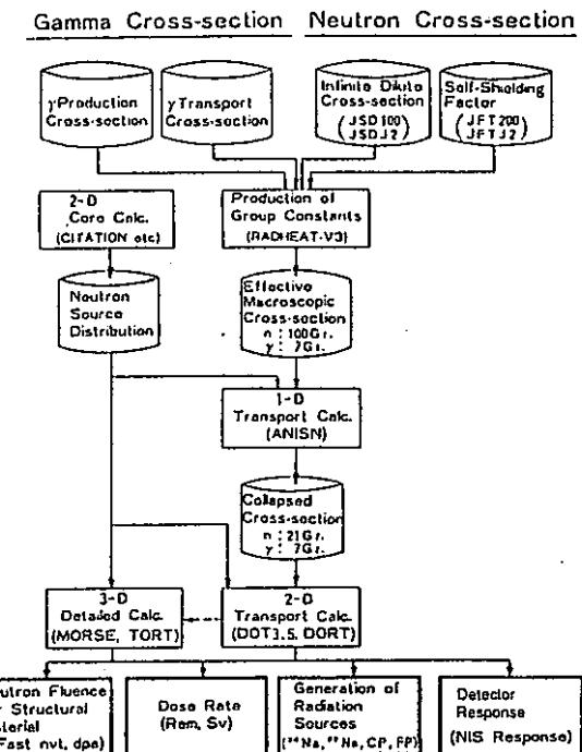
Fig. 4 Schematic Flow Diagram for the Shielding Analysis FBR Design
