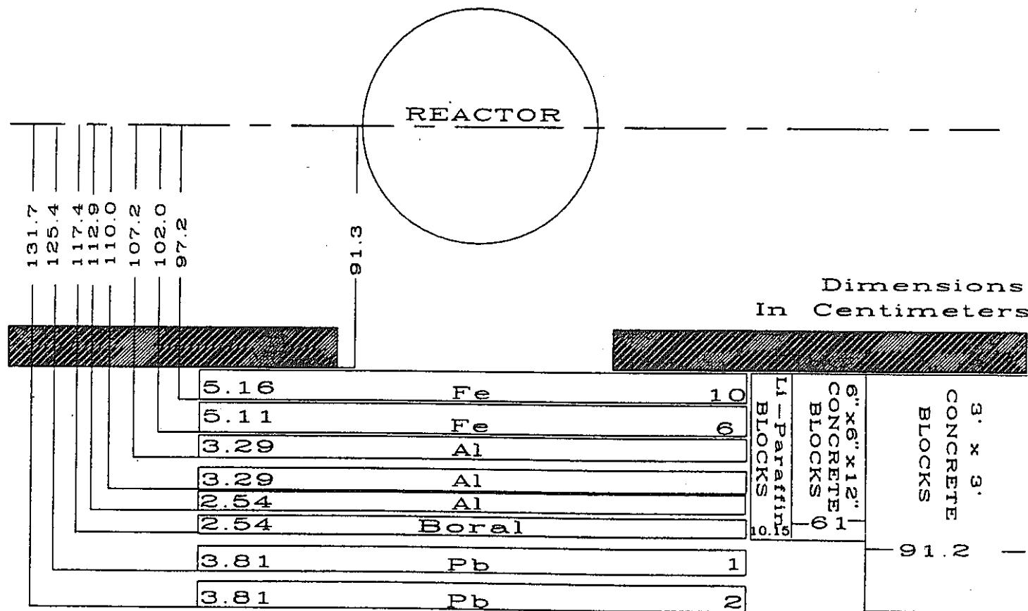
Figure 2. Schematic of SM-0 (Fe + Al + Boral) Item IA plus lead.
