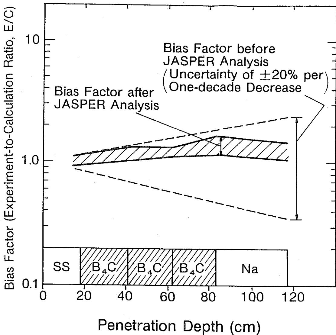
Fig. 7 Comparison of Calculation Uncertainty between before and after JASPER Analysis
