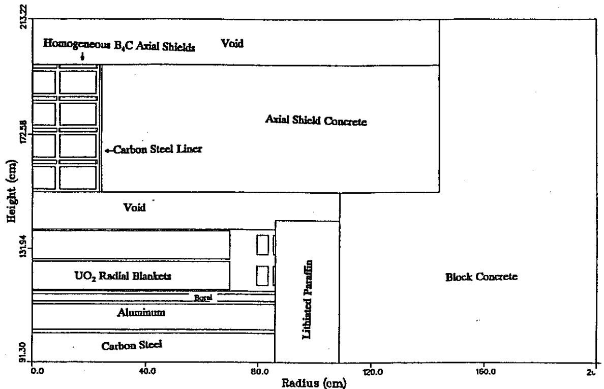
Fig. 1. Axial Shield Experiment 2-D Calculational Geometry Model for Case 1.
