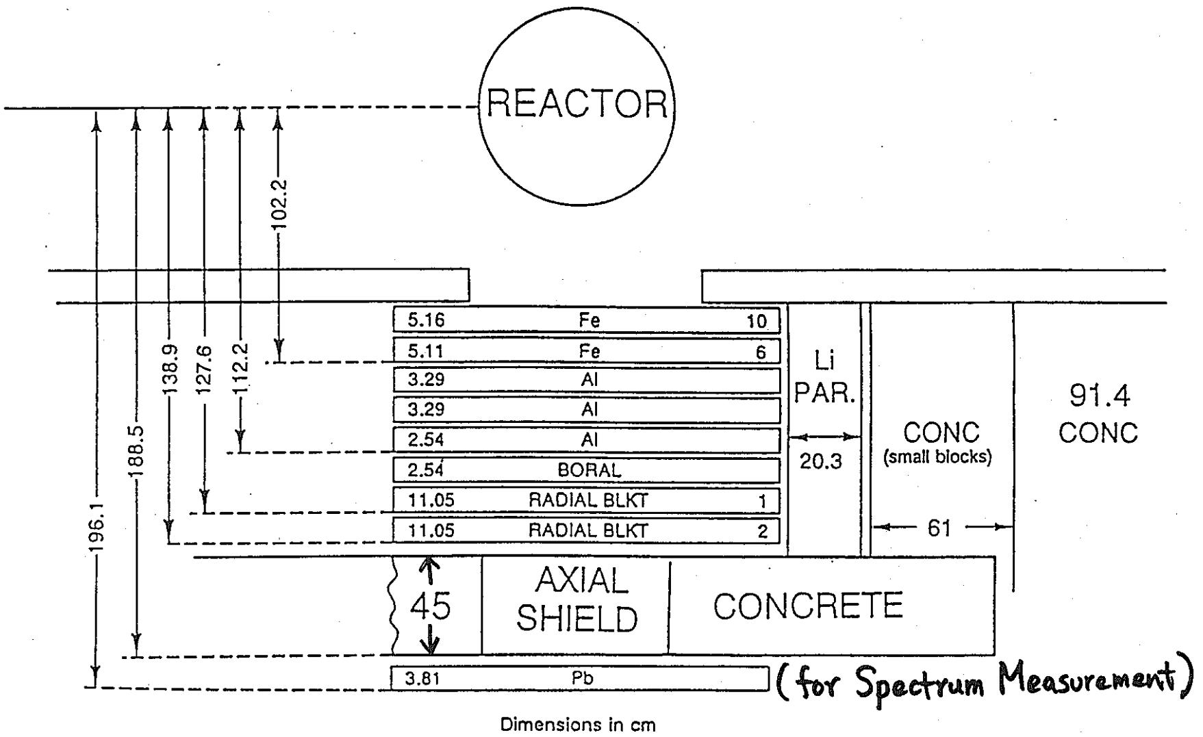
Fig. Schematic of the Axial Shield Mockup + Pb Slab
