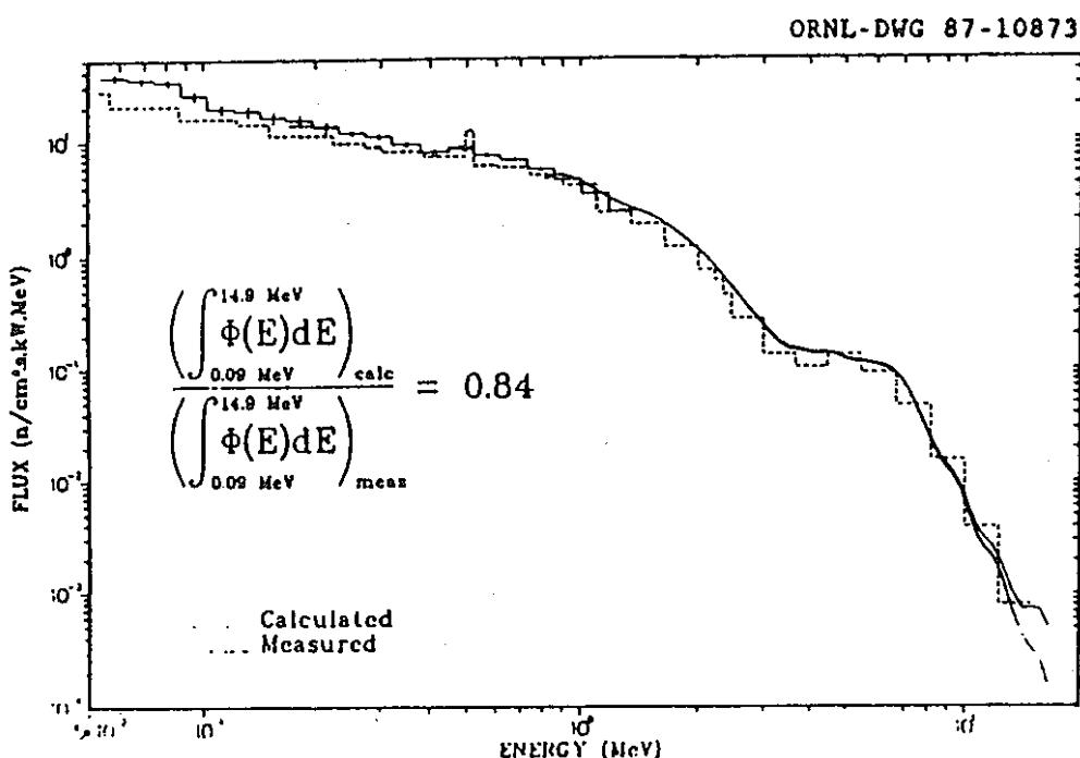
Fig. 7. Calculated versus measured  $E > 0.05$  MeV neutron spectra on centerline 63.2 cm behind Configuration VI.F.
