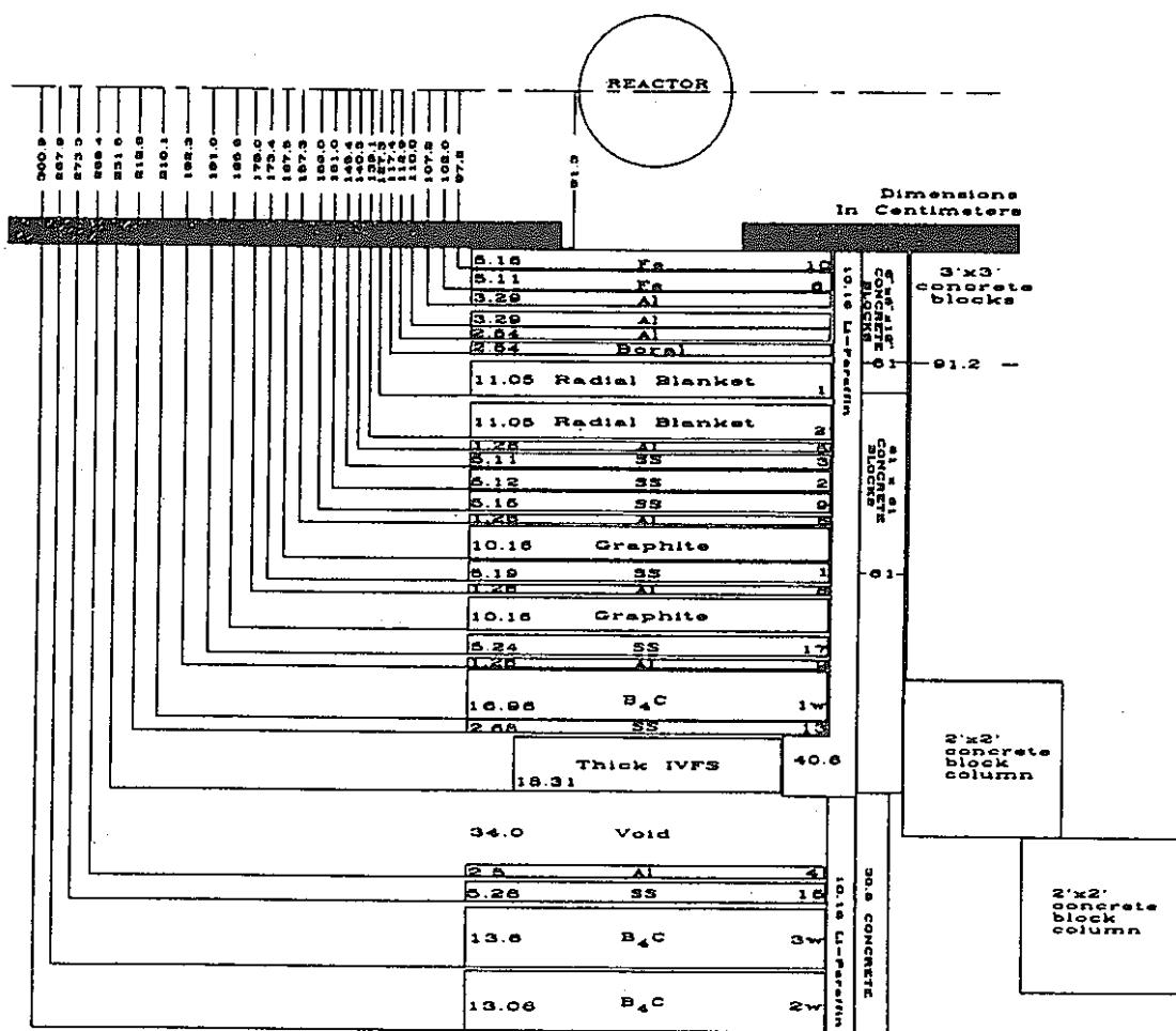
Figure 44A. Schematic of SM-1 plus shield mockup for Item IIP (Note: This mockup was used for measurements with the fission chamber in the void and at 0.7 and 30 cm behind mockup).
