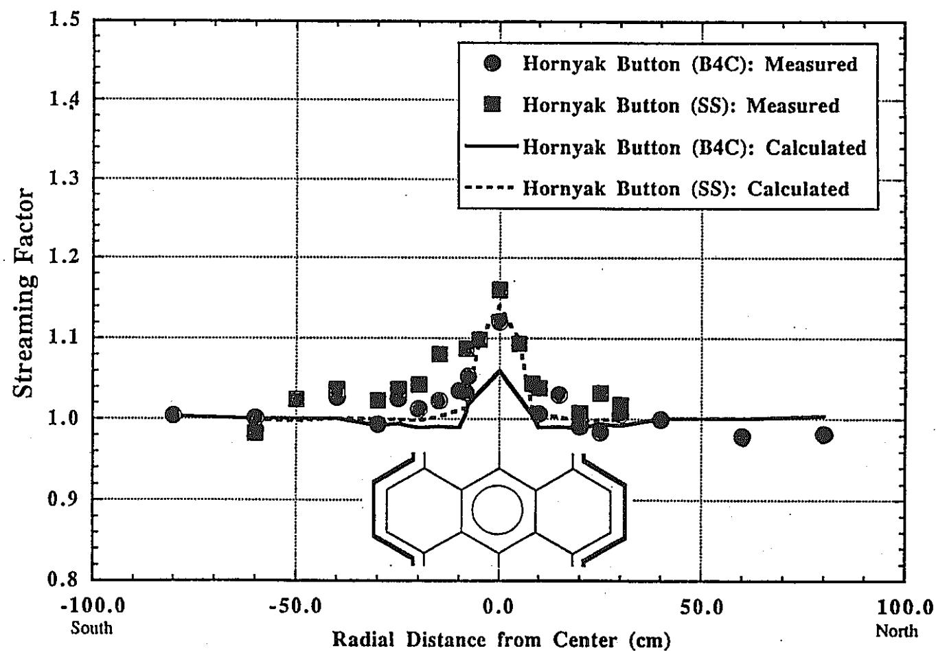
Radial Distributions of Streaming Factors derived from Hornýak Button Responses
