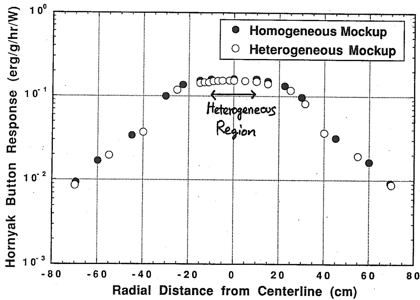
**Fig. Dose Rate Profile for Hornayak Button Measurements along Horizontal Traverse**
