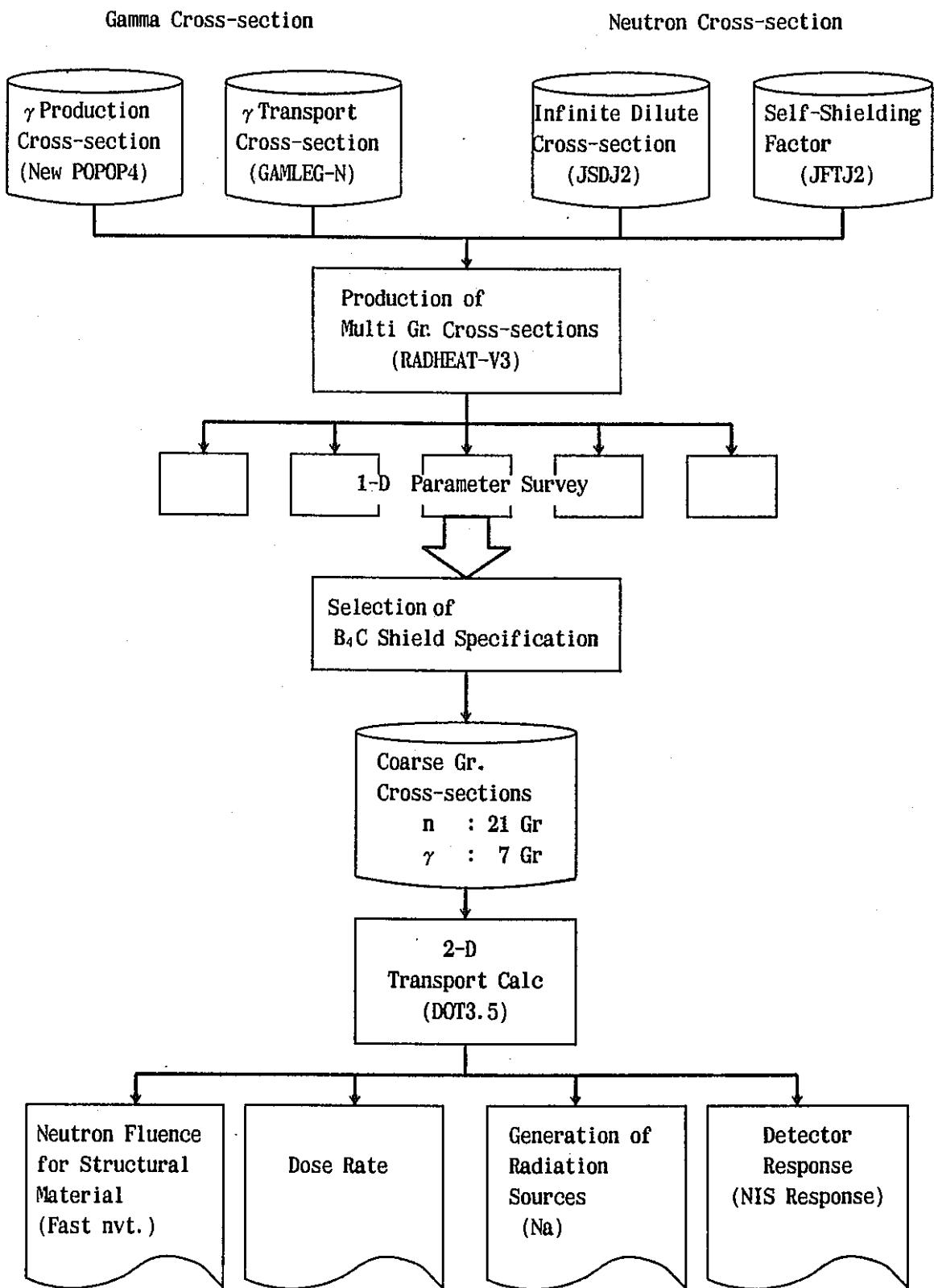
Fig. 2. Schematic Flow Diagram of Shielding Design
