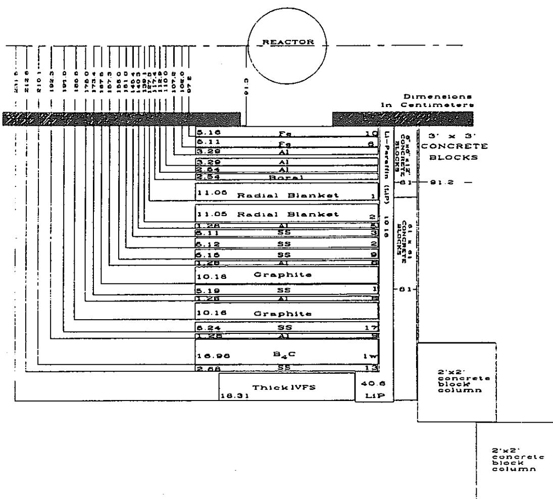
Figure 33. Schematic of SM-1 plus shield configuration for Item II I.
