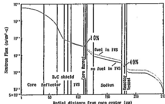
Fig. 6. Radial traverse of fast neutron flux
