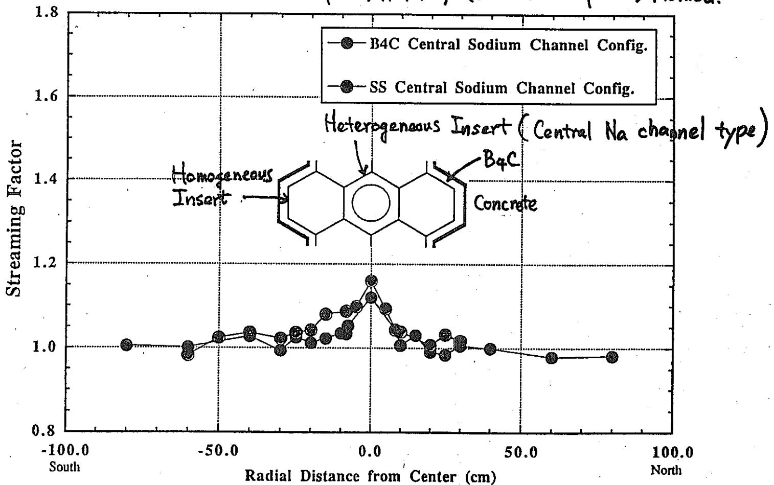
Radial Distributions of Streaming Factor derived from Measured Hornyak Button Responses
