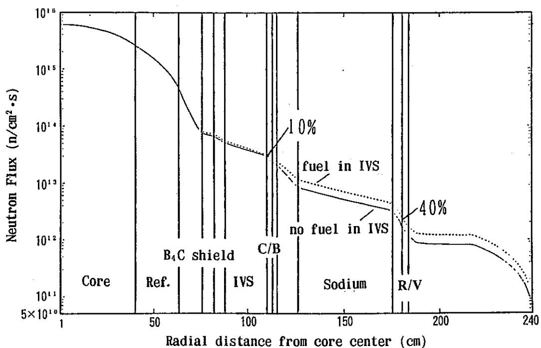
Fig. 6. Radial traverse of total neutron flux
