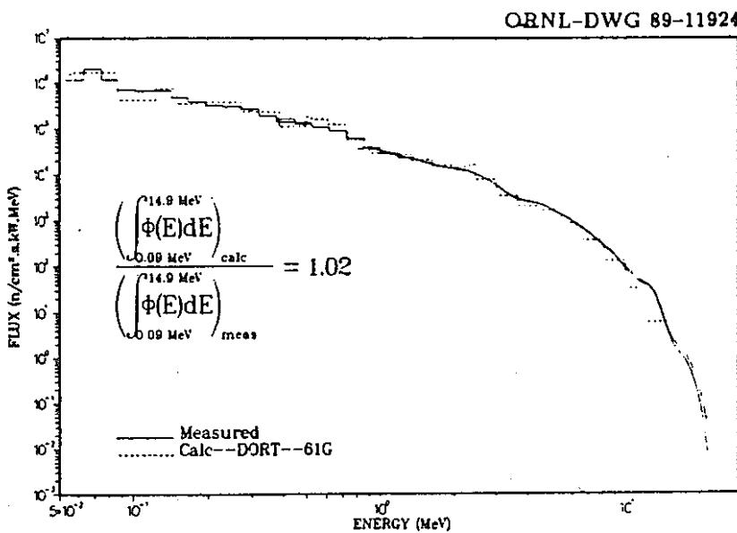
Fig. 6. Calculated versus measured  $E > 0.05$  MeV neutron spectrum behind Configuration III.
