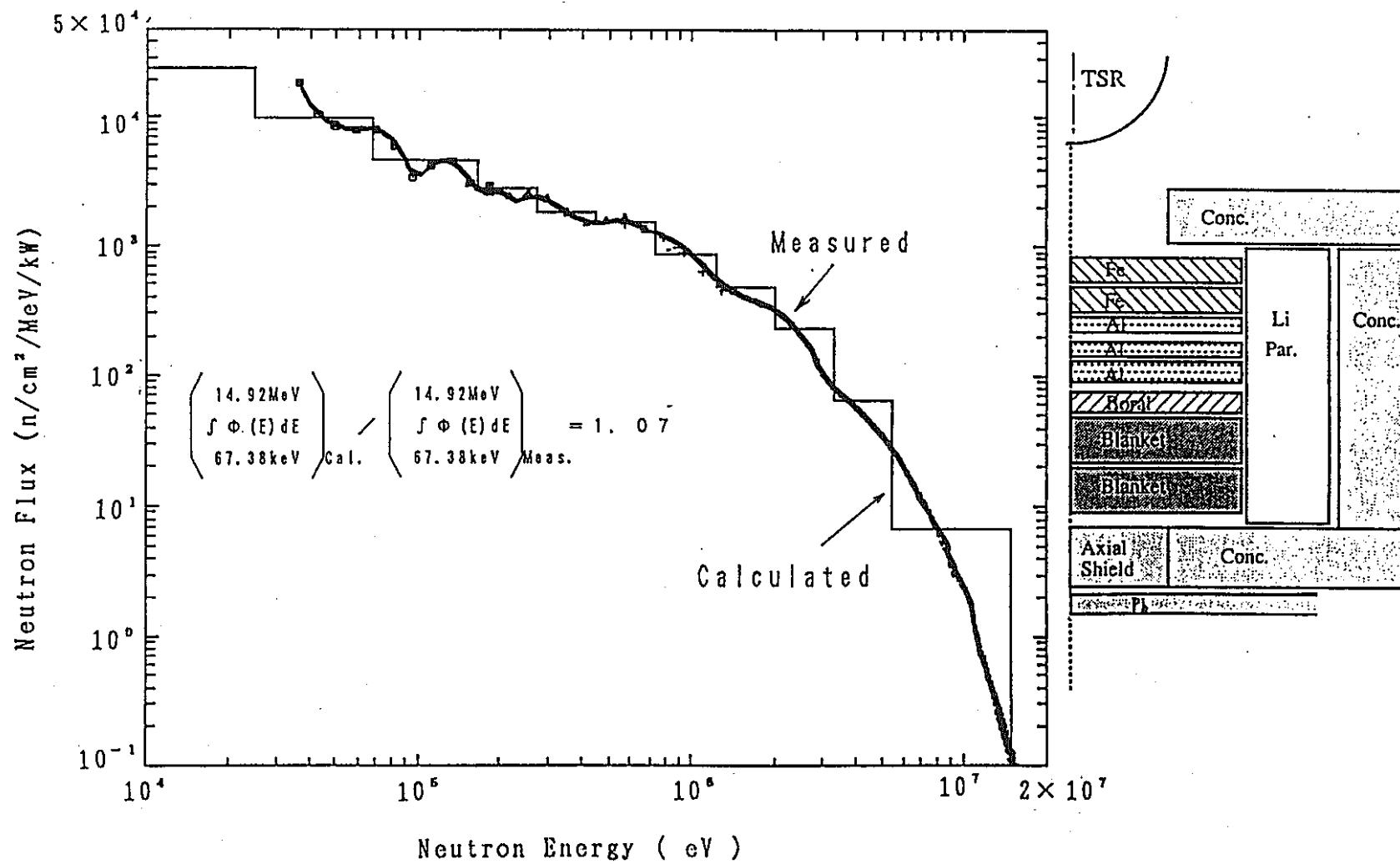
Fig. Comparison of Measured and Calculated Fast Neutron Spectra
