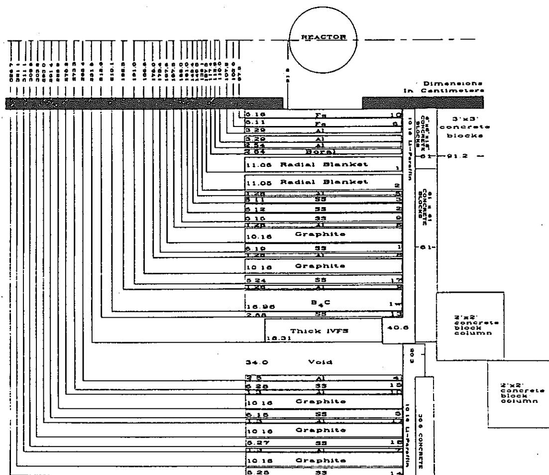
Figure 45A. Schematic of SM-1 plus shield configuration for Item IIQ
