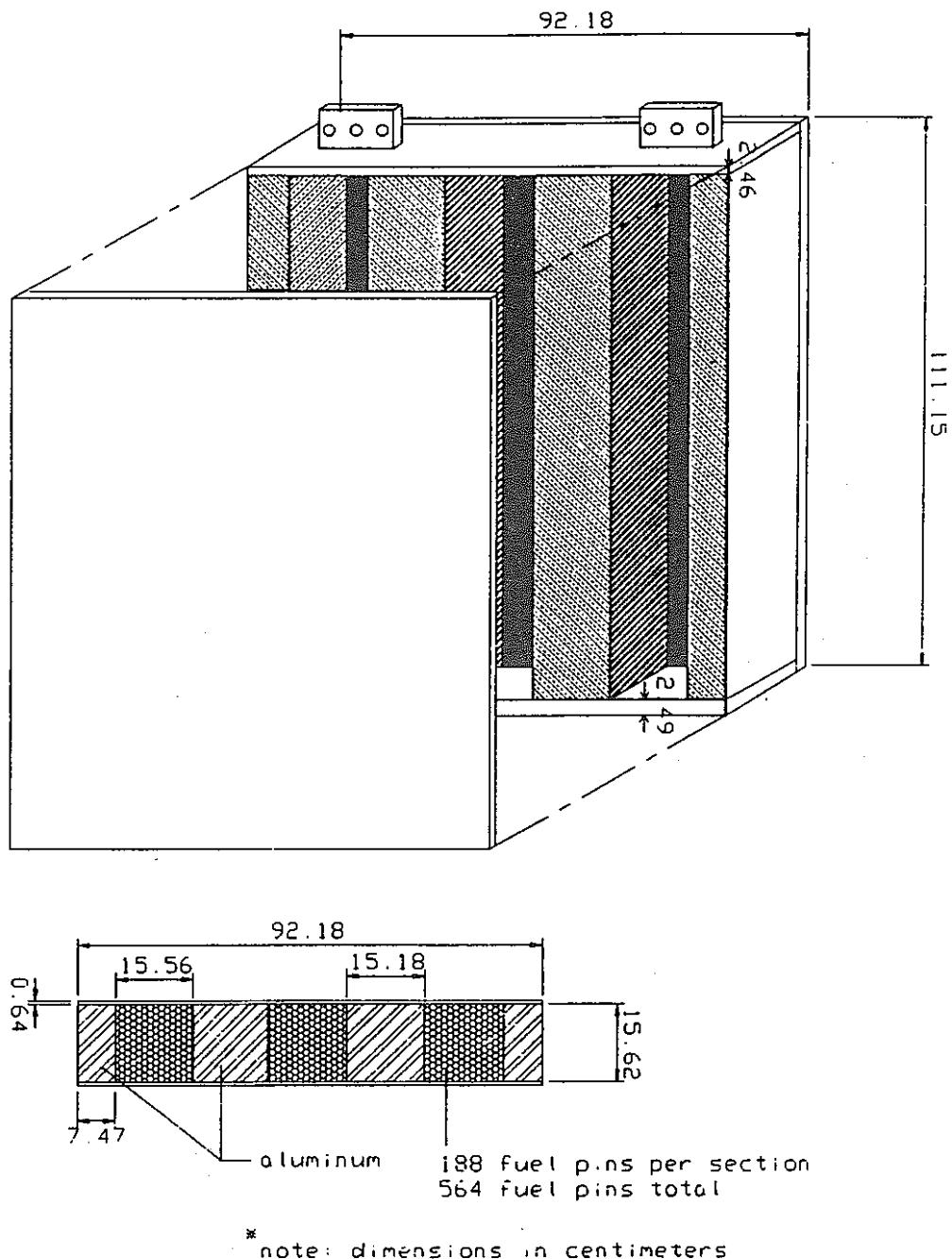
Figure 9. Schematic of heterogeneous IVFS mockup (slab #2).
