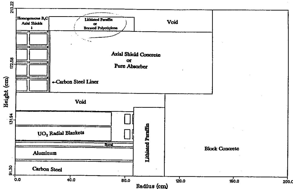
Fig. 5. Axial Shield Experiment 2-D Calculational Geometry Model for Cases 6 through 9.
