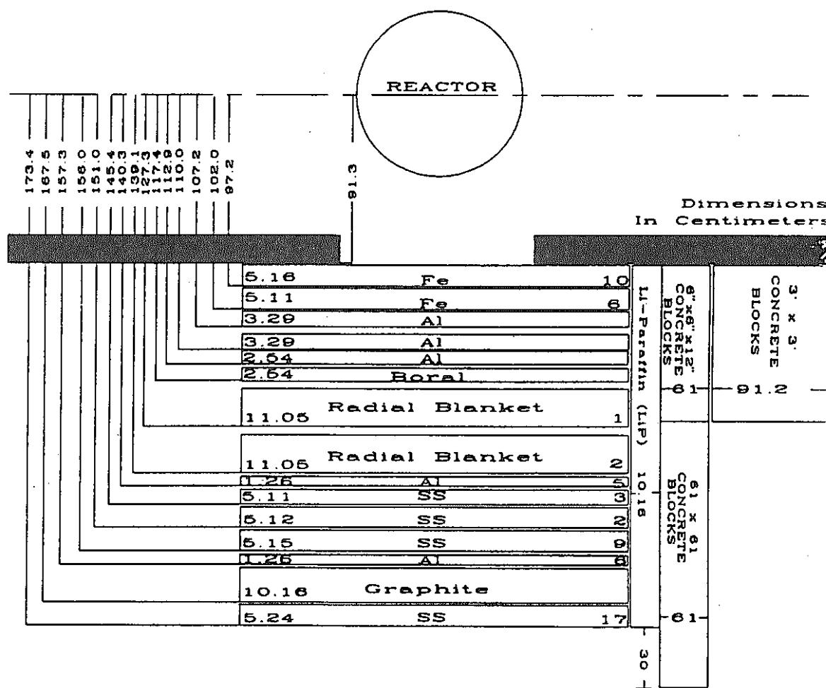
Figure 17. Schematic of SM-1 plus shield configuration for Item II A.
