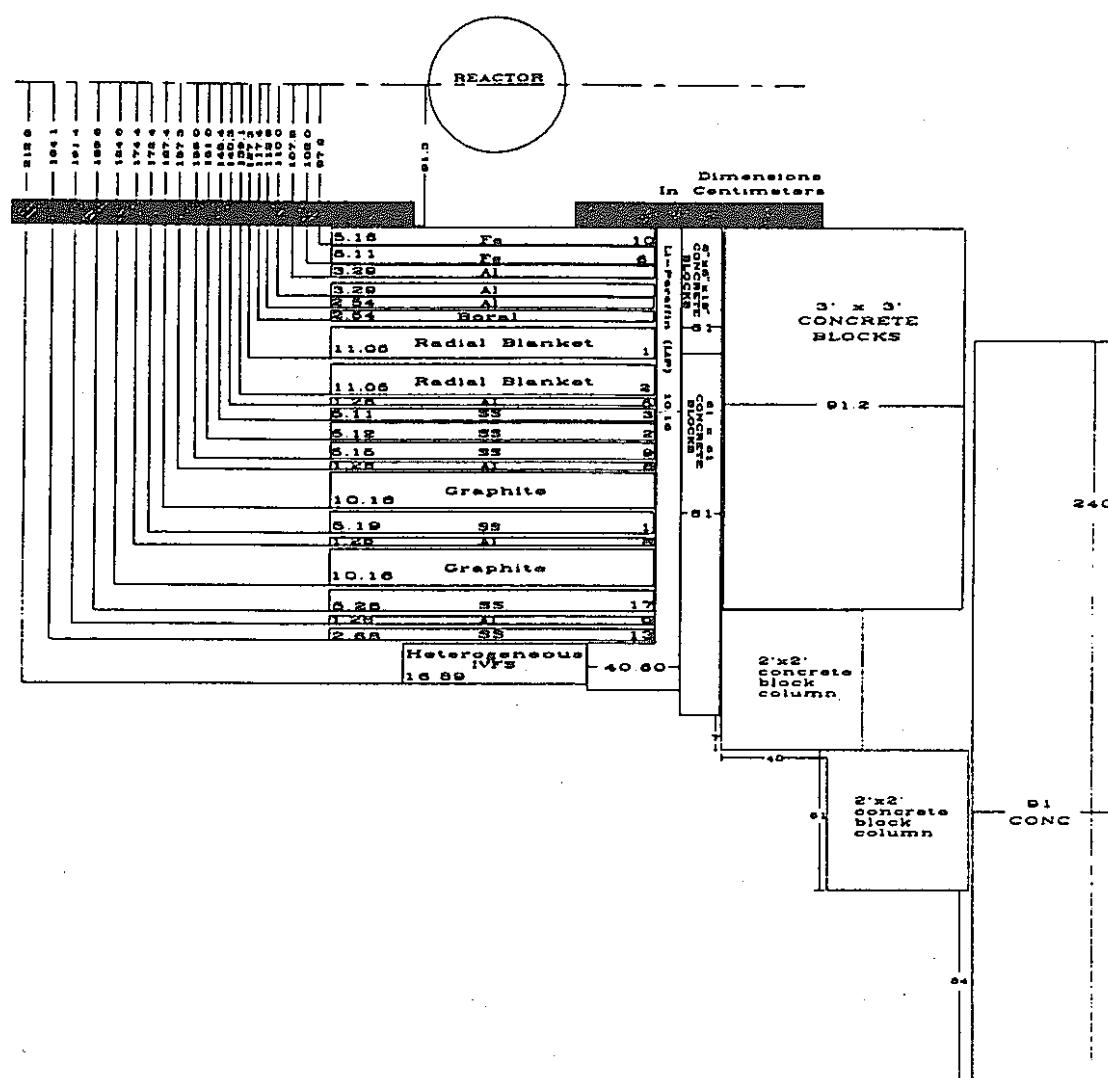
Figure 24. Schematic of SM-1 plus shield configuration for Item IID.
