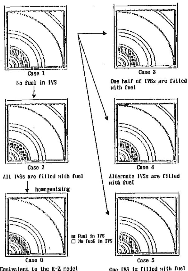
Fig. 8. Models for the 2D X-Y calculations by DOT3.5
