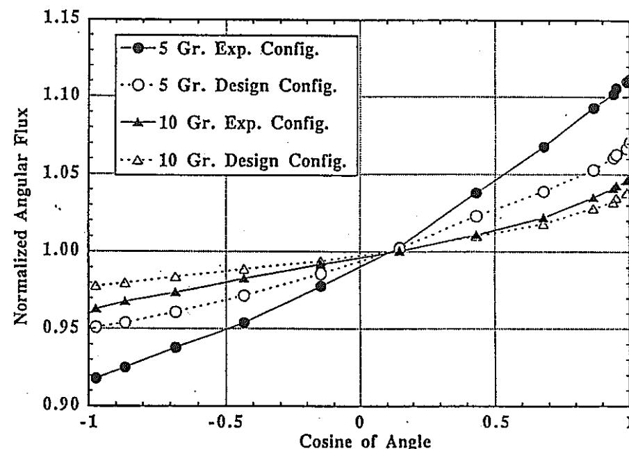
Angular Distribution of Incident Neutron Flux to Fission Gas Plenum Region
