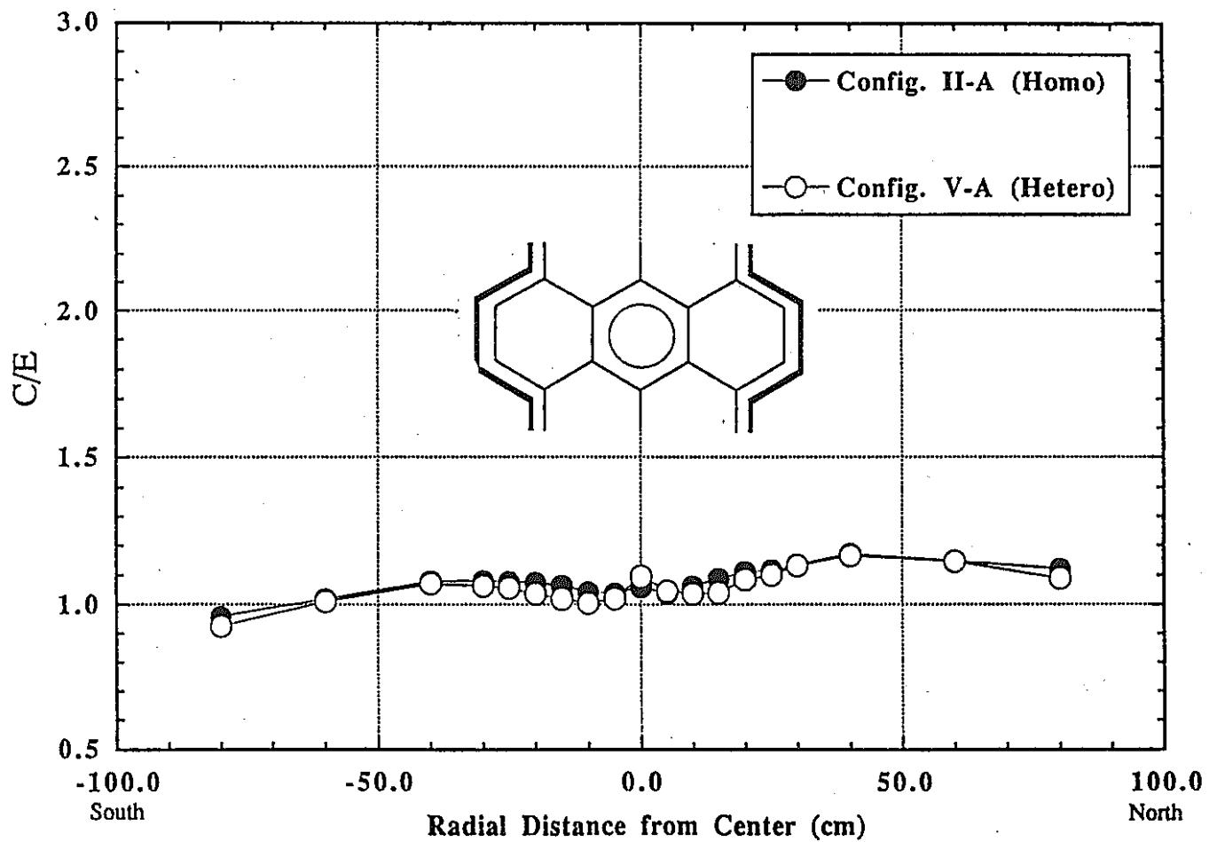
C/E Distributions of 5 inch Bonner Ball Response for B4C Type Axial Shield Configurations
