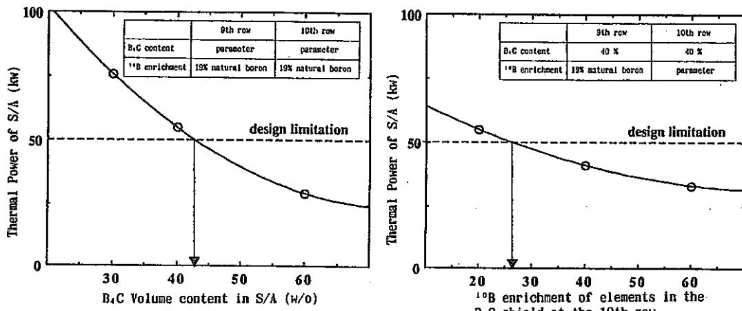
Fig. 3. Relationship between the thermal power of S/A in IVS and the B<sub>4</sub>C volume content in B<sub>4</sub>C shield S/A
