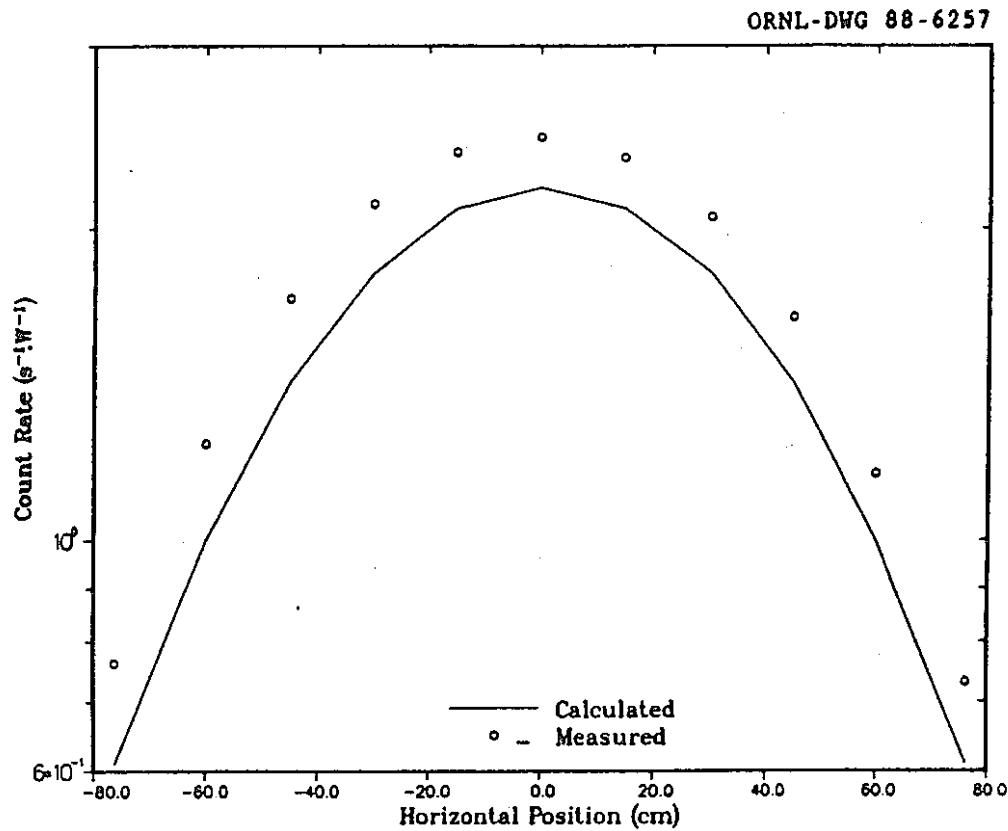
Figure 28. Comparison of calculated and measured 5-in. Bonner ball count rates for a horizontal traverse 30 cm behind Configuration VI.F (C/E range: 0.80-0.89).
