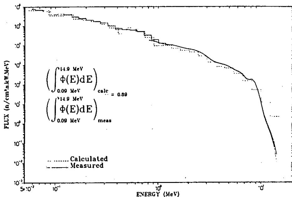
Figure 3. Calculated versus measured  $E > 0.05$  MeV neutron spectra on centerline 178.8 cm behind Configuration I.A.
