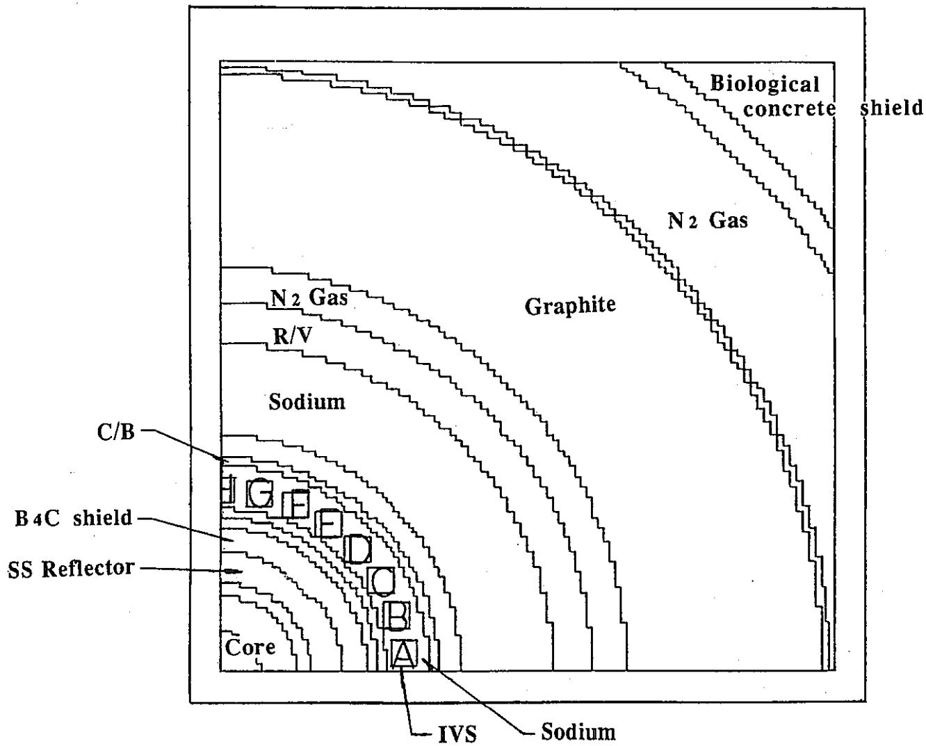
Geometry modeling for X-Y calculations
