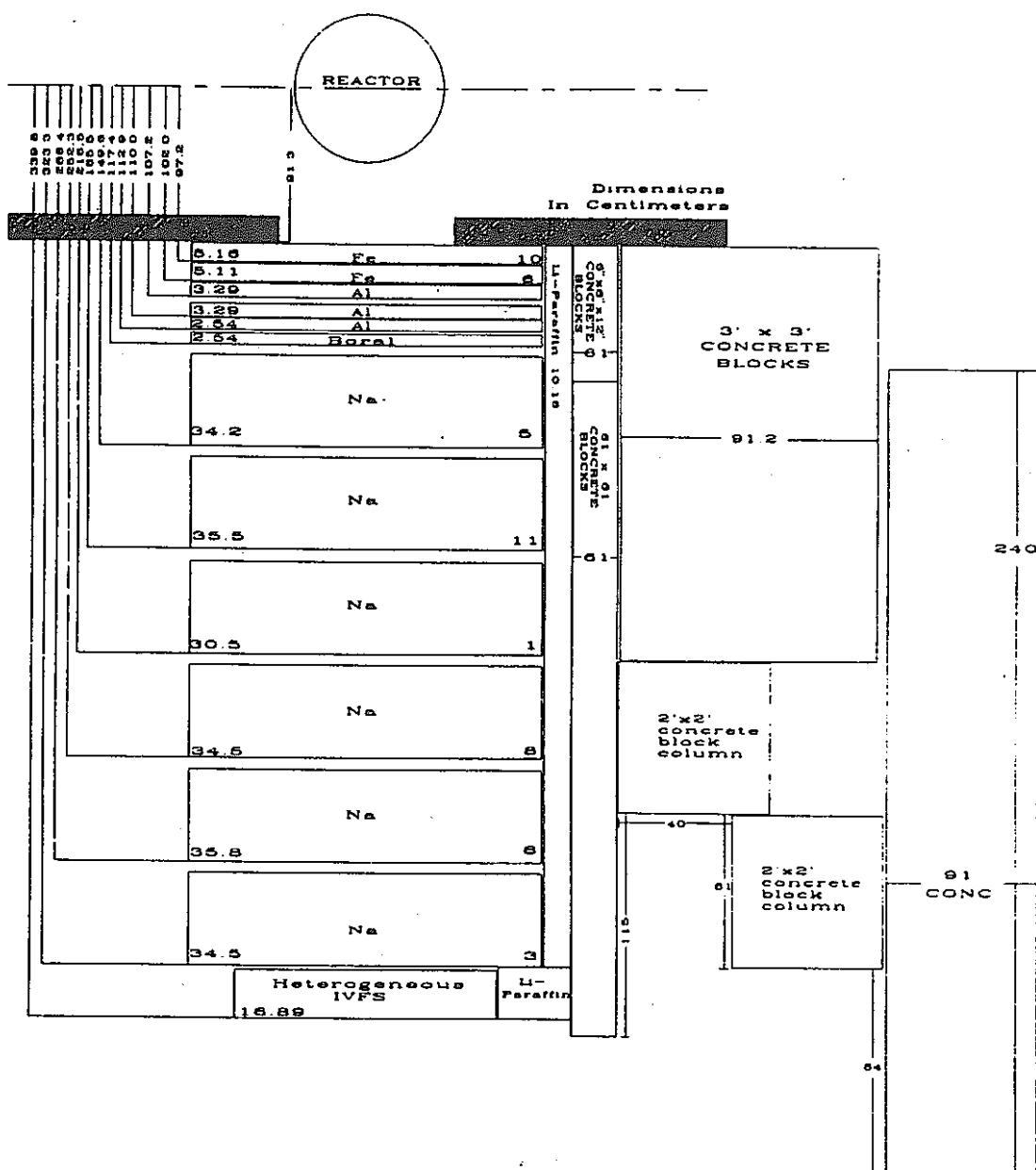
Figure 46. Schematic of SM-2 plus shield configuration for Item IIIA.
