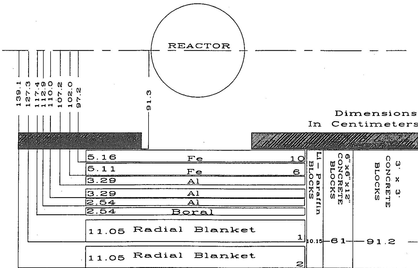
Figure 3. Schematic of SM-1 (Fe + Al + Boral + radial blankets) Item IB.
