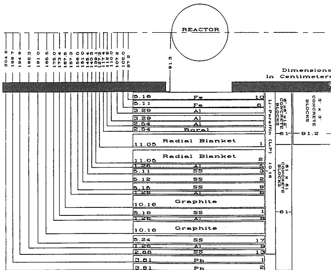
Figure 18. Schematic of SM-1 plus shield configuration for Item IIB plus lead.
