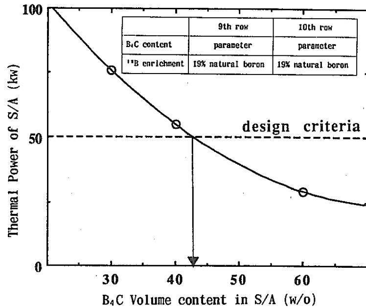
Fig. 3. Relationship between the thermal power of S/A in IVS and the B<sub>4</sub>C volume content in B<sub>4</sub>C shield S/A
