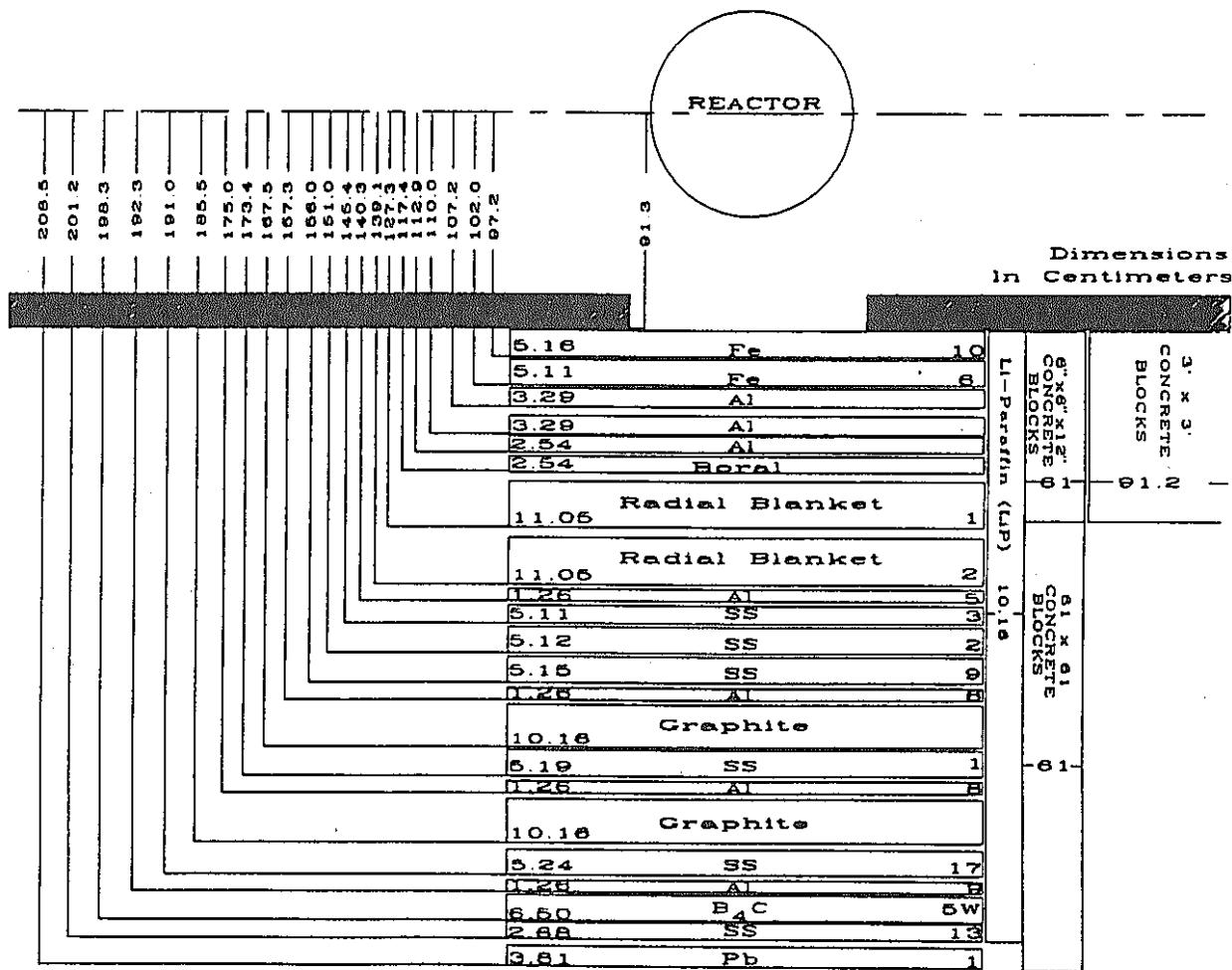
Figure 26. Schematic of SM-1 plus shield configuration for Item IIF plus lead.
