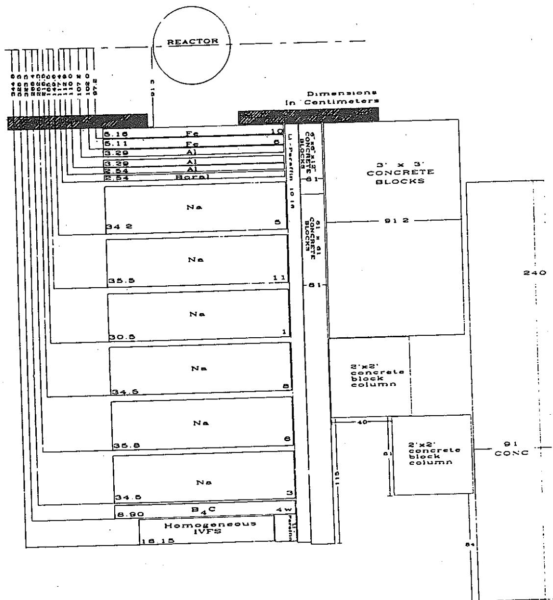
Figure 50. Schematic of SM-2 plus shield configuration for Item IIIE.
