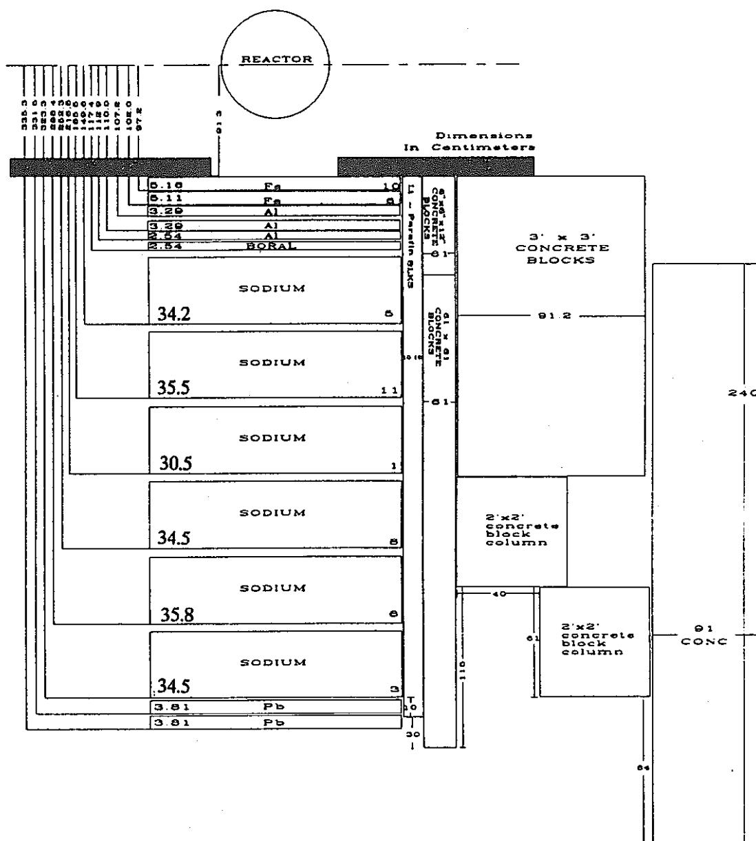
Figure 5. Schematic of SM-2 (Fe + Al + Boral + sodium) plus lead.
