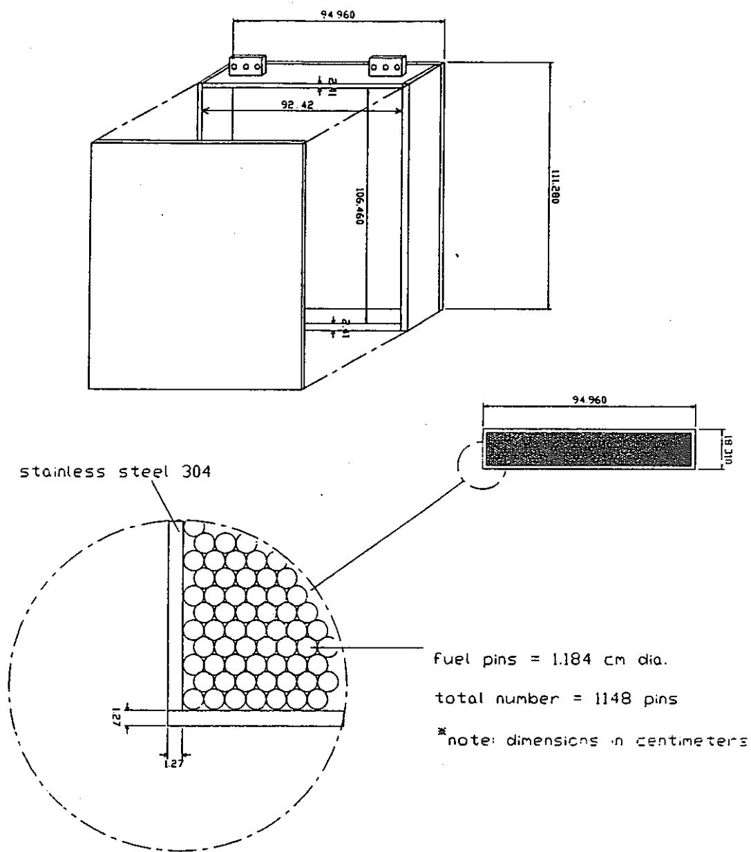
Figure 8. Schematic of thick IVFS mockup (slab #1).
