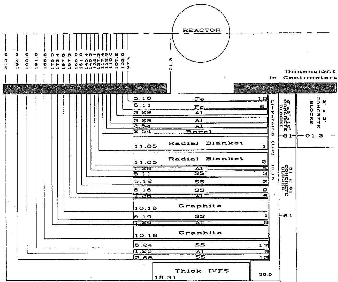
Figure 21. Schematic of SM-1 plus shield configuration for Item IIC.
