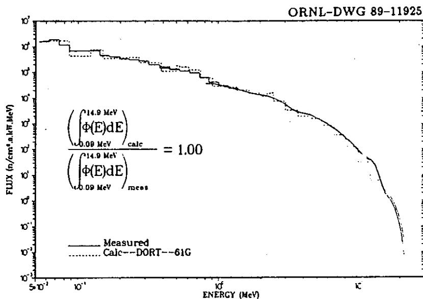
Fig. 7. Calculated versus measured  $E > 0.05$  MeV neutron spectrum behind Configuration V (no streaming correction).
